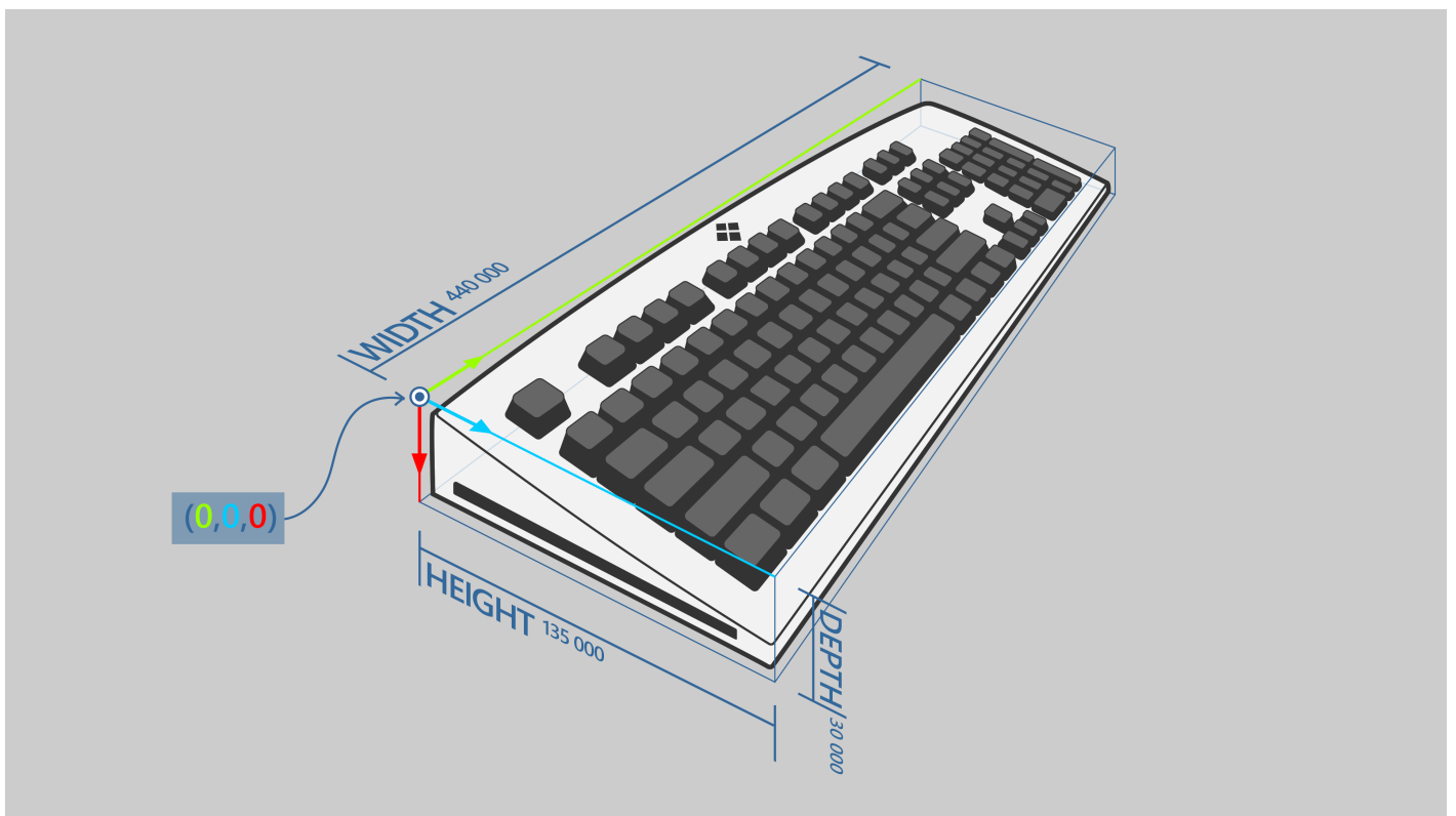
Figure 26.2: Keyboard with labeled dimensions and origin. Lamps exist beneath every key, the branding at the top/middle, and accent lighting along the left and right sides. Example sizes given for each dimension (in \mu\text{m} ).
