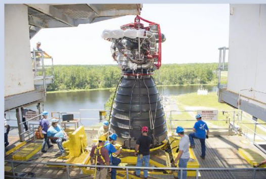
RS-25 Engine Being Installed on the A-1 Test Stand at Stennis Space Center in Preparation of a Hot Fire Test
