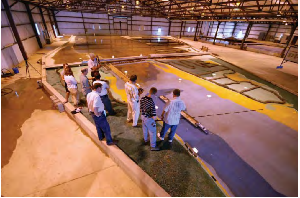
Model of Lock and Dam 25
