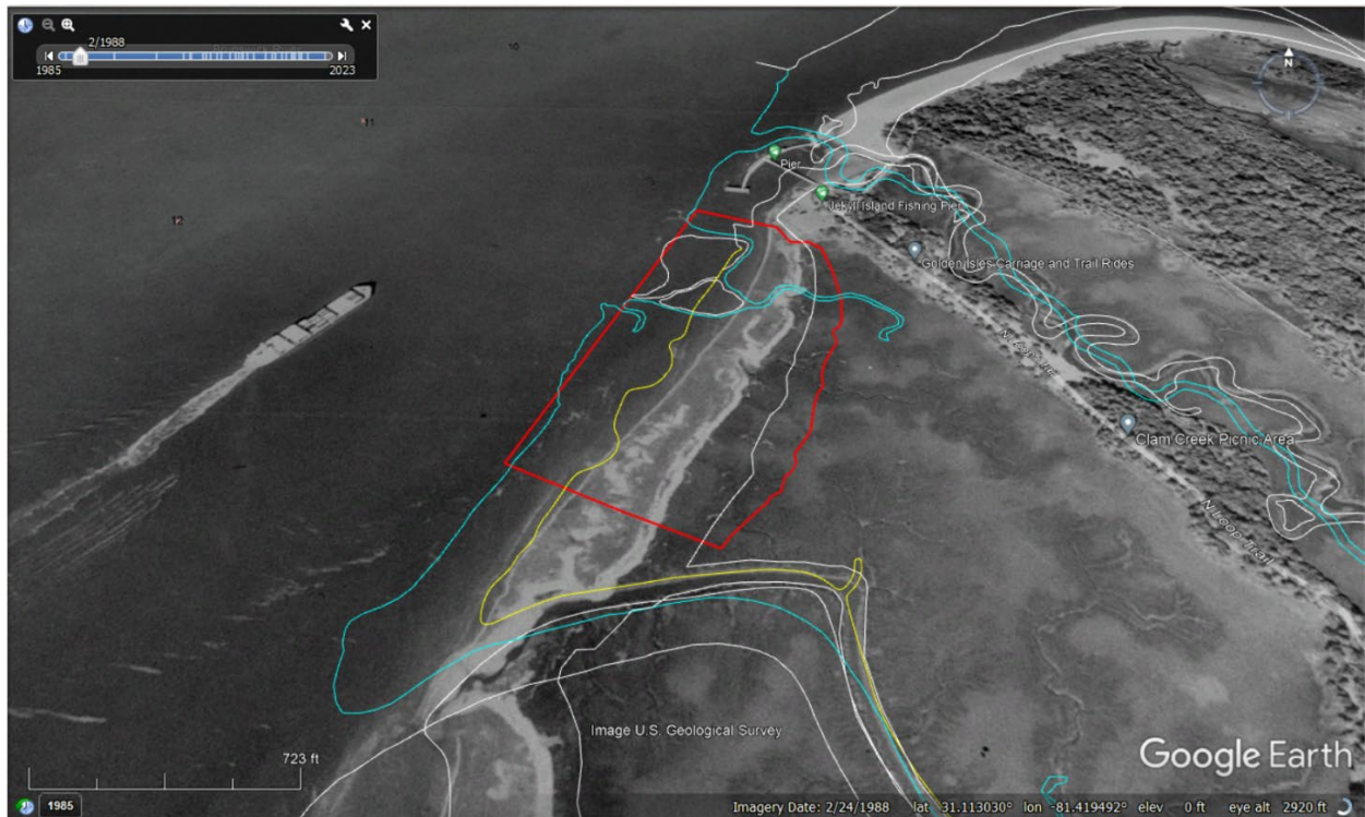
Figure 3. 1988 aerial imagery of the proposed placement location. The proposed placement polygon is in red. The blue line is historical shoreline from 1855, and the yellow is historical shoreline from 1933 (G-WRAP, 2023).
