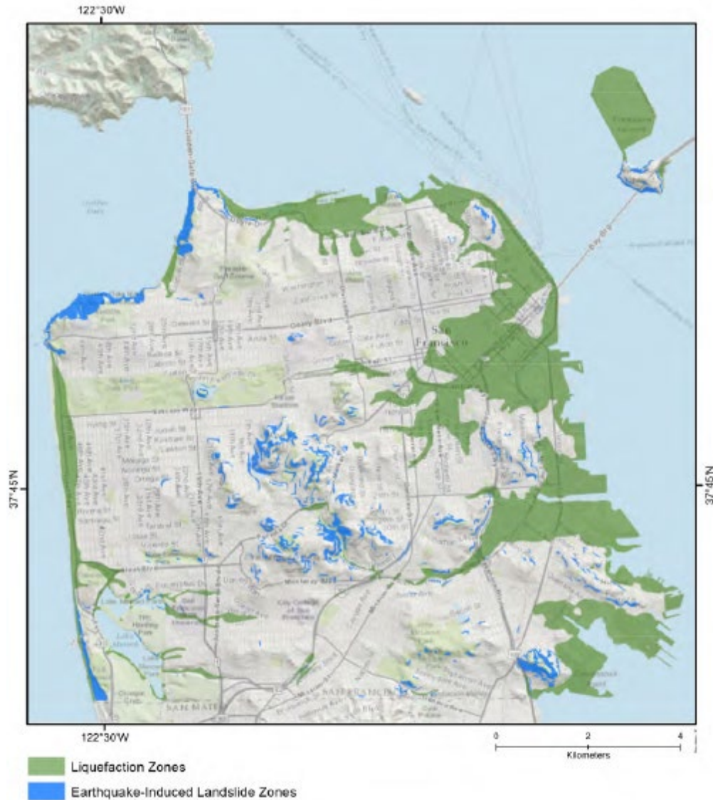
Figure B-6: California Geological Survey’s Seismic Hazard Zones Map Showing Zones of Liquefaction and Earthquake-Induced Landslides
