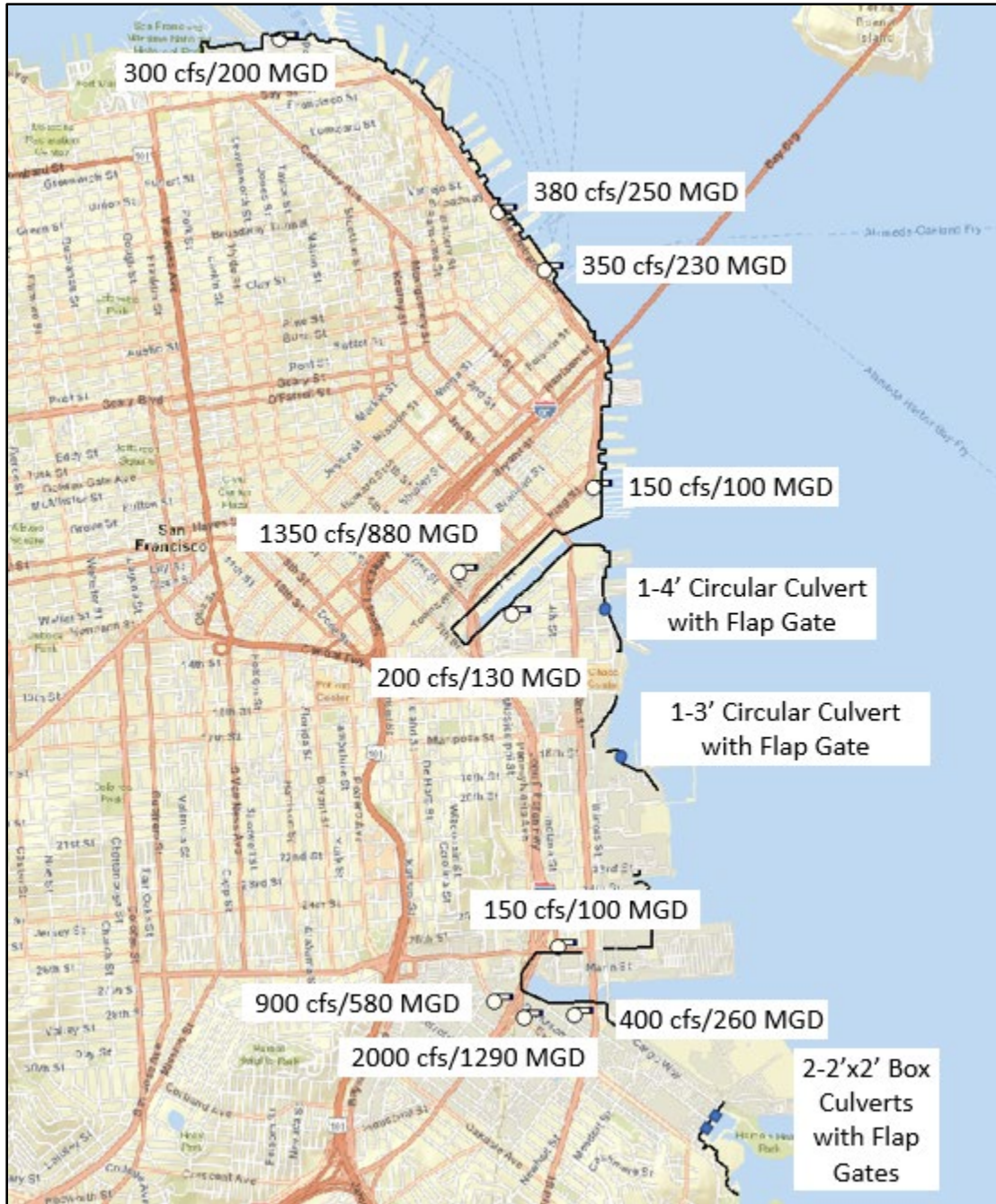
Figure B.1.4-29: Alternative G First Action General Locations and Sizing of Interior Drainage Features
