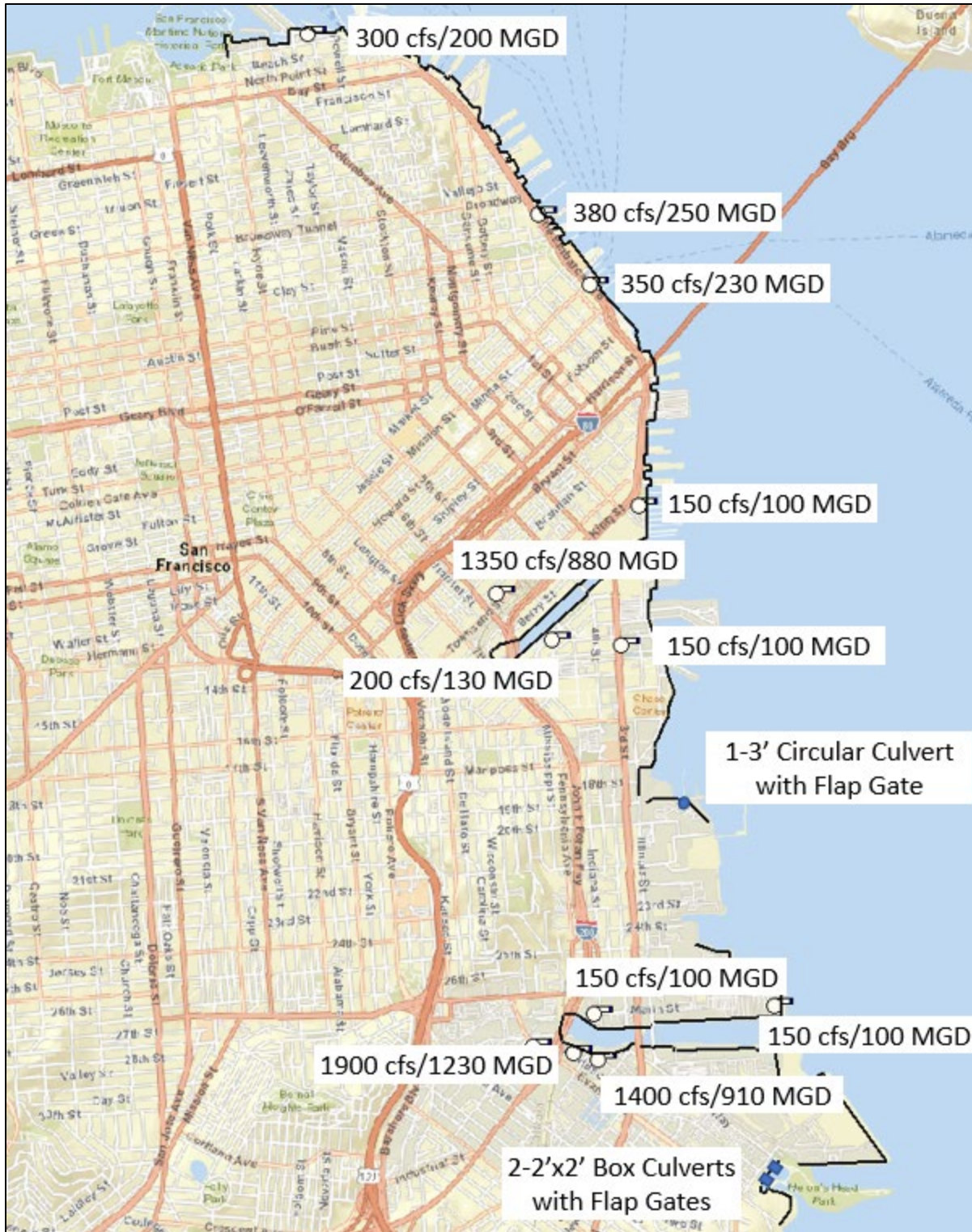
Figure B.1.4-26: Alternative E General Locations and Sizing of Interior Drainage Features
