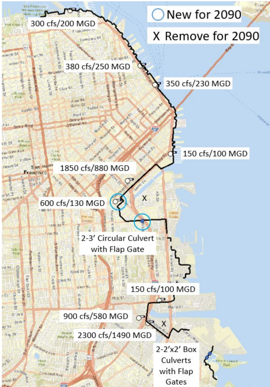
Figure B.1.4-30: Alternative G Second Action General Locations and Sizing of Interior Drainage Features
