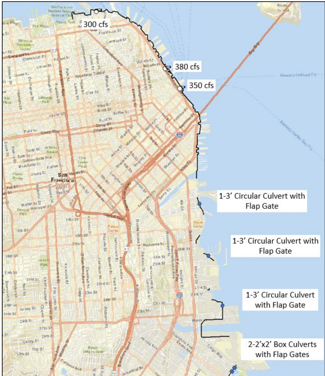
Figure B.1.4-27: Alternative F First Action General Locations and Sizing of Interior Drainage Features
