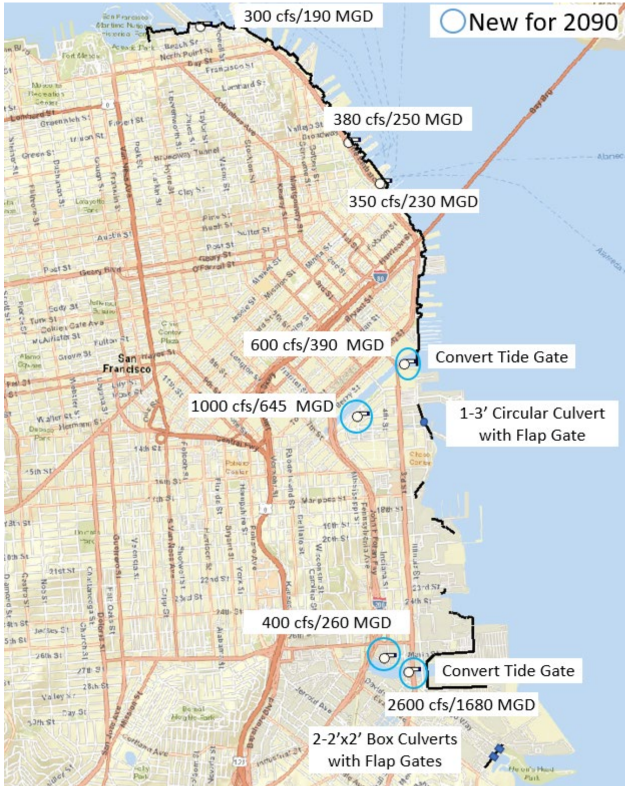
Figure B.1.4-28: Alternative F Second Action General Locations and Sizing of Interior Drainage Features
