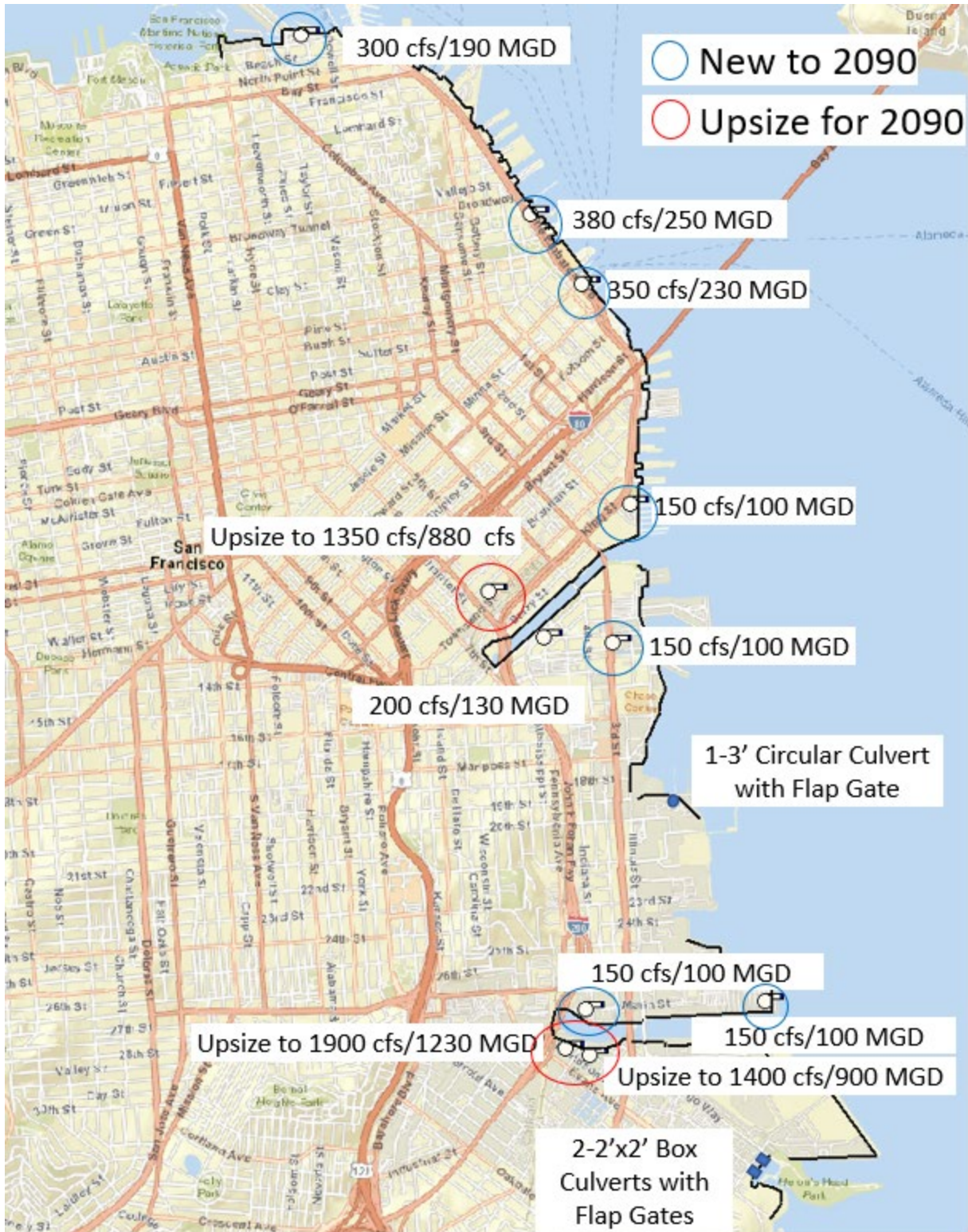
Figure B.1.4-25: Alternative D Second Action General Locations and Sizing of Interior Drainage Features
