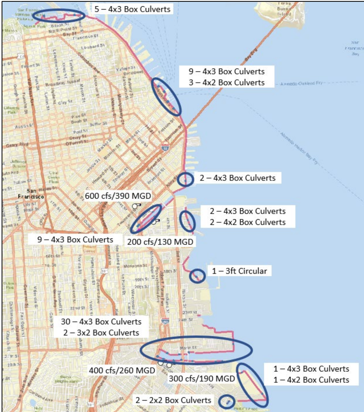
Figure B.1.4-24: Alternative D First Action and Alternative C General Locations and Sizing of Interior Drainage Features
