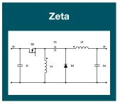
$$D = \frac{-V_{out} + V_f}{-V_{out} + V_f + V_{in}}$$
