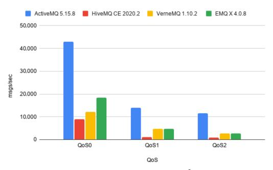
**Figure 8.** Projected message rate (msgs/sec) of scalable brokers at 100% system CPU usage in the local evaluation environment.
