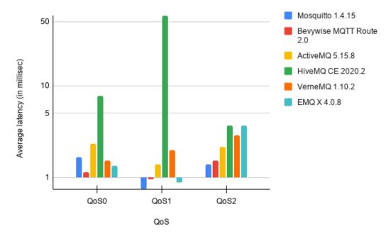
**Figure 7.** A comparison of average latency of all scalable and non-scalable brokers in the local evaluation environment.
