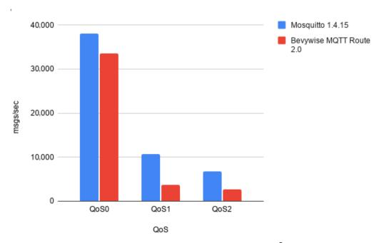
**Figure 6.** Projected message rate (msgs/sec) of non-scalable brokers at 100% process CPU usage in the local evaluation environment.
