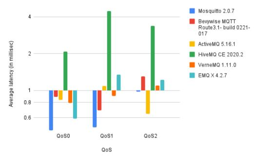
**Figure 10.** A comparison of average latency of all scalable and non-scalable brokers in the cloud evaluation environment.
