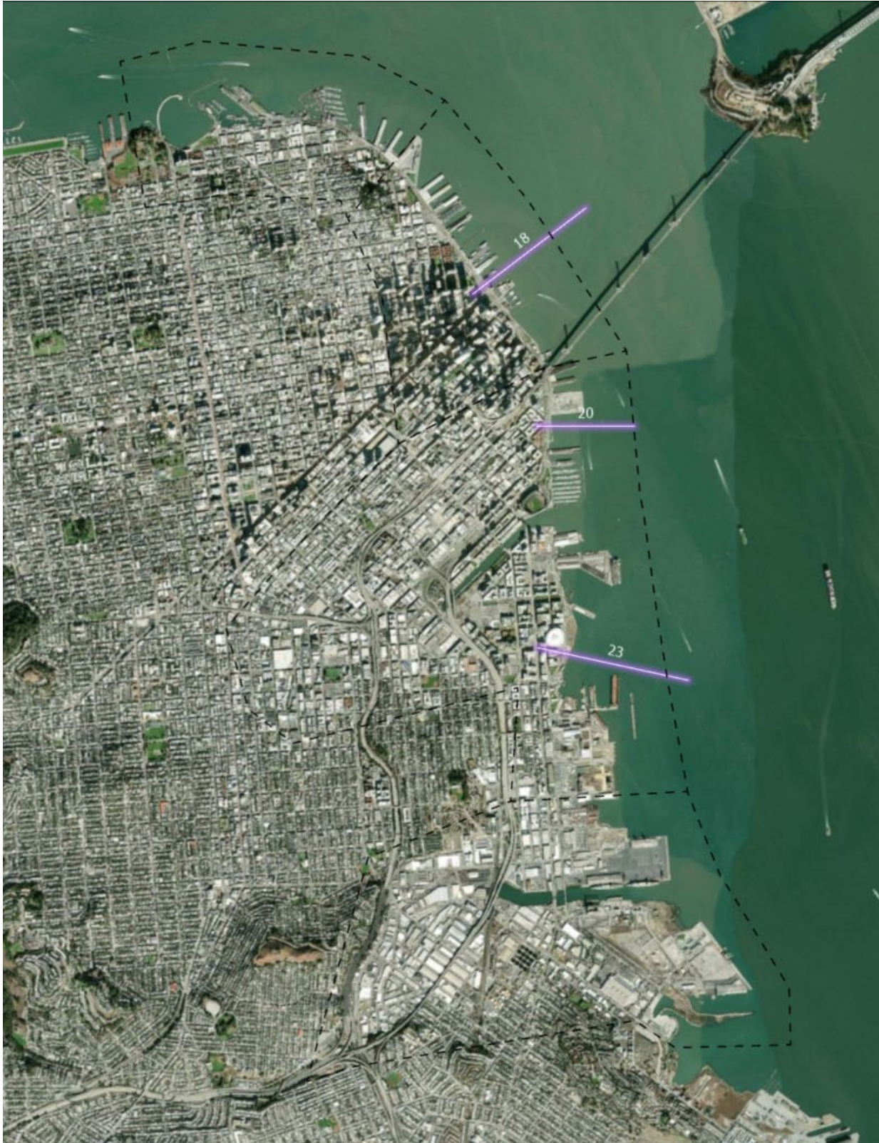
Figure B.1.3-1: Transect Locations for Wave Overtopping Analysis (FEMA Analysis Transect Locations)
