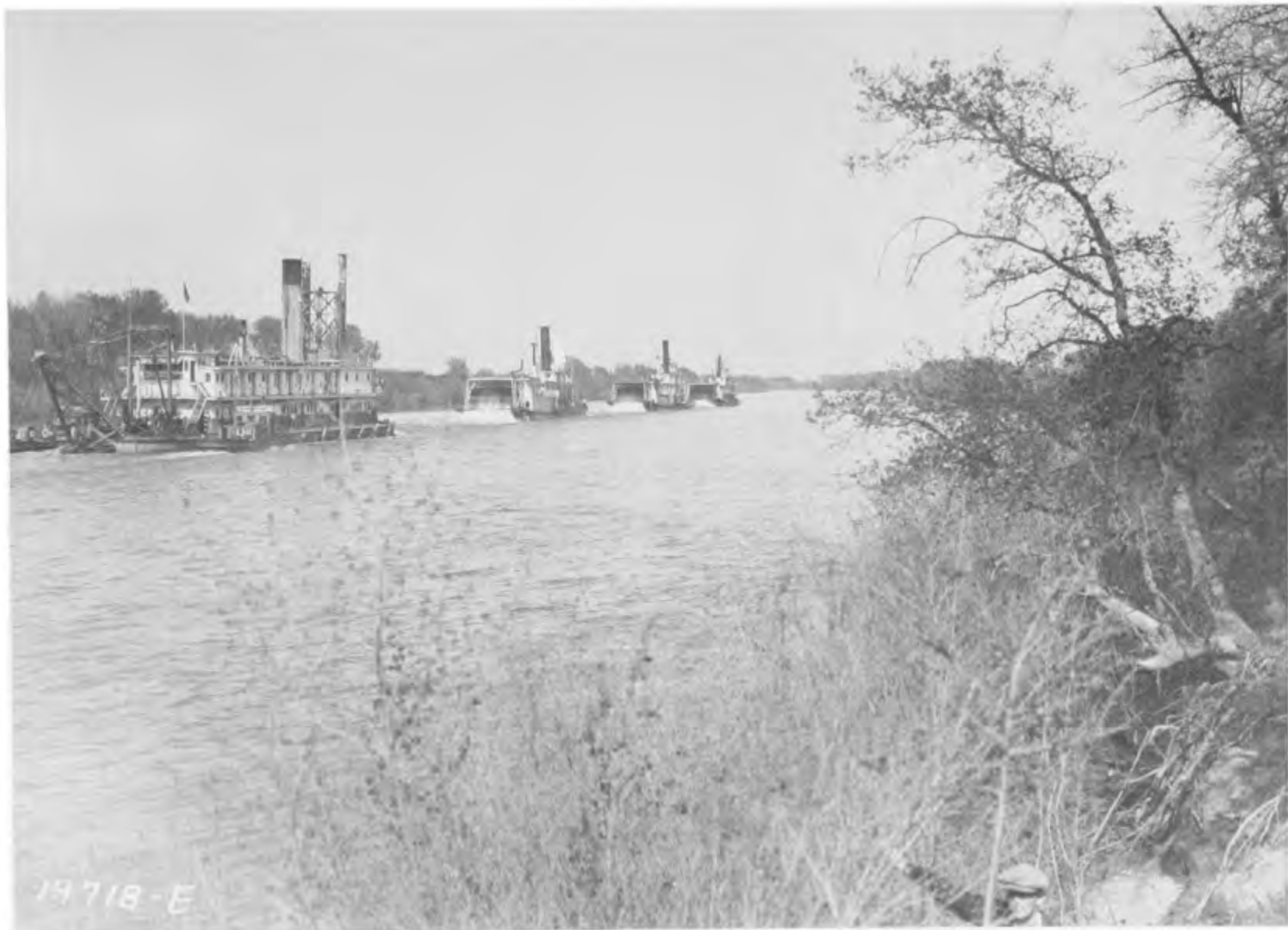
PADDLE WHEEL BOATS TOW A DREDGE UP THE SACRAMENTO RIVER — AUGUST 1927 — NOTE THE DREDGE TENDER ALONGSIDE.
