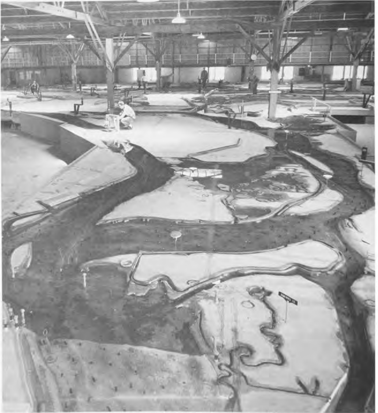
YOU'RE LOOKING AT THE SACRAMENTO RIVER ON THE LEFT AND THE SAN JOAQUIN ON THE RIGHT AND YOU'RE STANDING IN THE MIDDLE OF SUISUN BAY. WITH THIS DELTA ADDITION TO THE CORPS OF ENGINEERS' WORKING MODEL OF SAN FRANCISCO BAY, PROBLEMS OF POLLUTION, WATER QUALITY, NAVIGATION, AND OTHER ITEMS CAN BE STUDIED FOR SOLUTIONS LEAST HARMFUL TO THE ENVIRONMENT.
