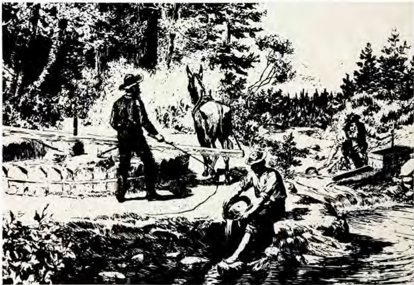
In this composite early gold-mining scene, one miner operates a horse-powered arrastra, a second pans ore, and a third works with a rocker.
