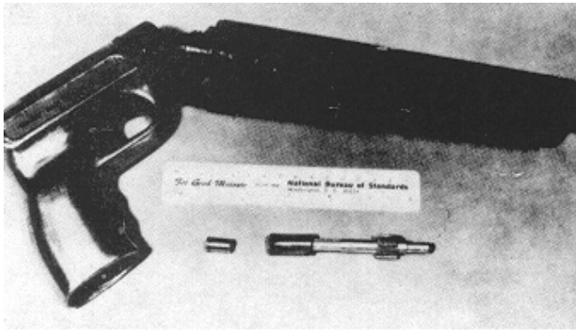
Figure 2-36. Windsor probe apparatus showing the gun, probe, and blank cartridge
