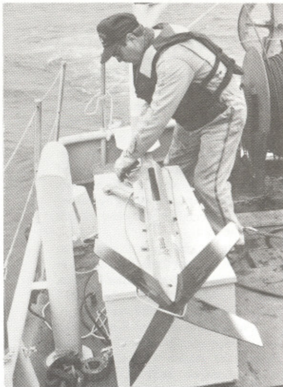
Ken Cinker, deckhand from the Duluth vessel yard, connects a cable to one of the sonar "fish" on the deck of the survey boat David Boyd . A variety of equipment including side-scan sonar and underwater television was used to locate the barrels on the bottom of Lake Superior.
