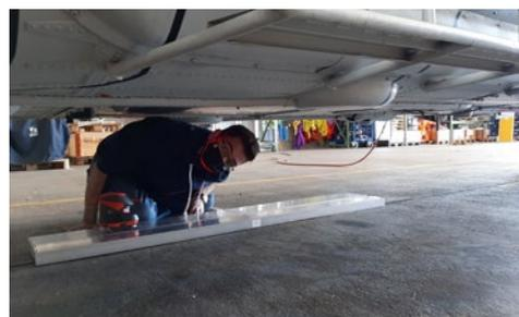
**Figure 4: Positioning of the sources under the helicopter.**
