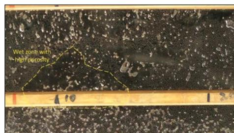
**Figure 6: Observation of wet zone in the debris bed formed after downward melt relocation.**
