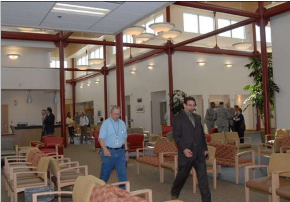
Guests view the inside of the Fort Richardson Health Clinic after a ribbon-cutting ceremony June 1. Dominant architectural design elements are exposed structural steel members, rounded walls, clerestory windows to allow maximum daylight exposure and an open floor plan with one expansive hallway.
