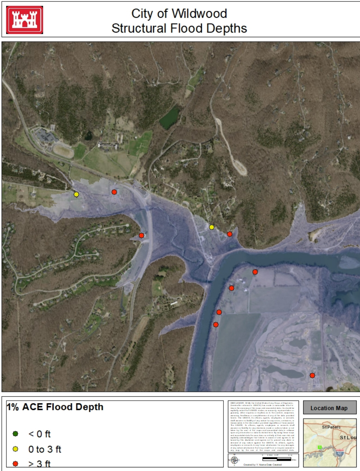
Figure 36. Wildwood Depth of Flooding Relative to 1st Floor Elevation
