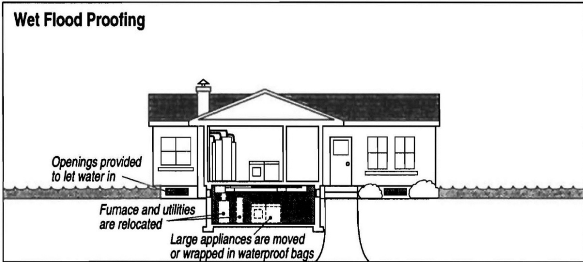
Figure 9. Wet Flood Proofing (Diagrammatic Detail/Section)
