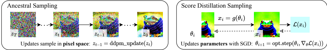
Figure 2: Comparison of 2D sampling methods from a text-to-image diffusion model with text “a photo of a tree frog wearing a sweater.” For score distillation sampling, as an example we use an image generator that restricts images to be symmetric by having \mathbf{x} = (\text{flip}(\theta), \theta) .
