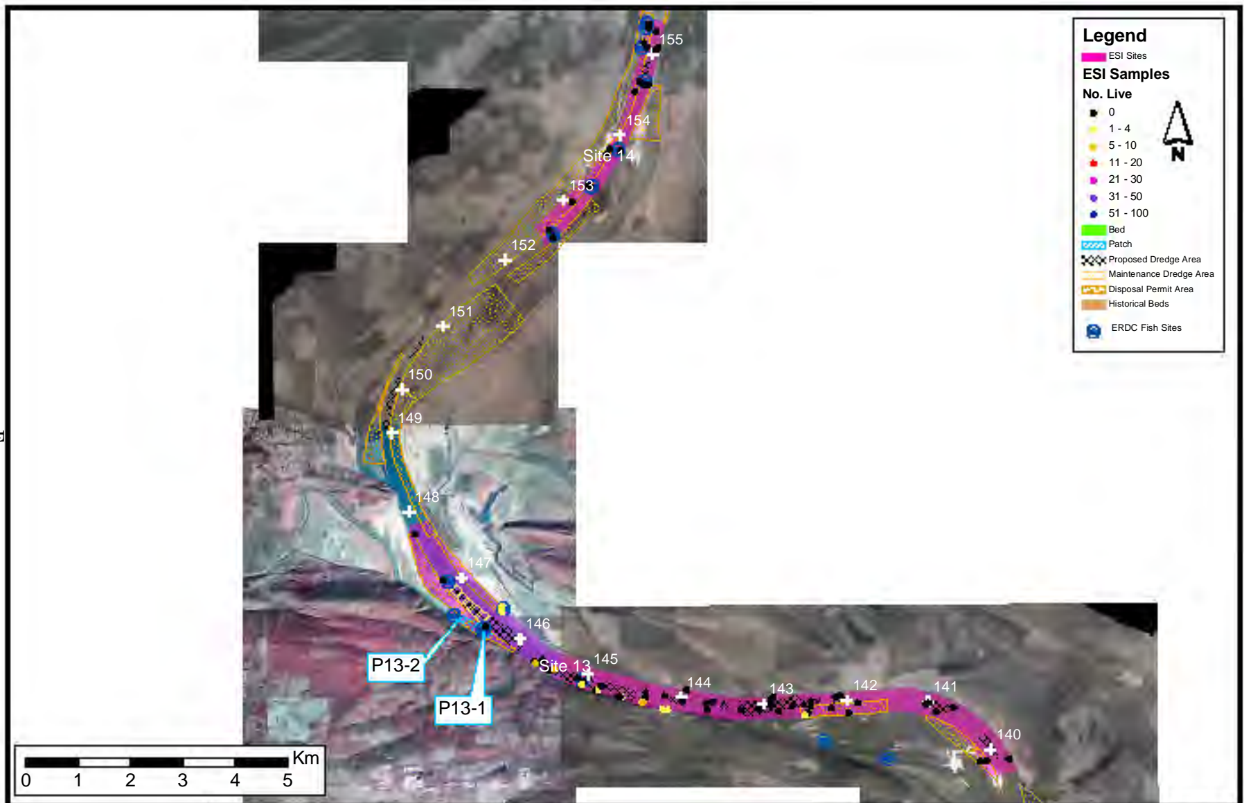
Figure 3-6. Proposed 12ft channel maintenance activity with respect to unionid beds and patches, Reach 3, Sites 13 to 14.
