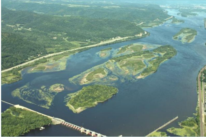
Figure 1.8. Aerial photo of Pool 6, 16 July 2010. Lock & Dam 6 discharge 49300 cfs. and elevation 643.6. The 1-foot drawdown was reached on 01 July. The large quantities of duckweed and algae that developed around the edge of exposed substrates made photo interpretation difficult for determining the amount of exposed substrate. Bottom right is the lock wall and the entrance to the marina that experienced the most difficulties with vegetation. Photo WDNR
