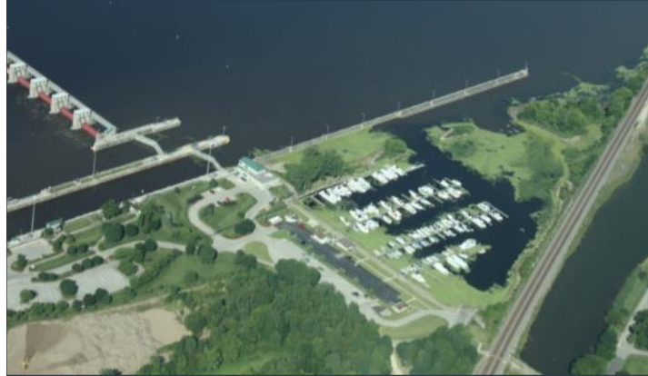
Figure 2.57. Marina, located in the SE corner of Pool 6 next to the locks. Dredging along the lock wall removed 500 cubic yards to improve access. In mid August floating mats of submersed aquatic plants were trapped in the marina as it is located in a dead end bay next to the lock chamber. A weed harvester removed over 200 tons (wet weight). WDNR
