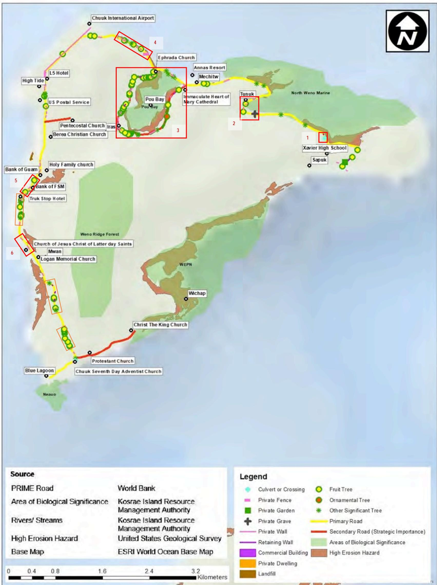
Figure 5-3: Key E&S sensitivities on Primary Road network – Chuuk (showing 'high' (red box) and 'medium' (orange box) sensitivities).
