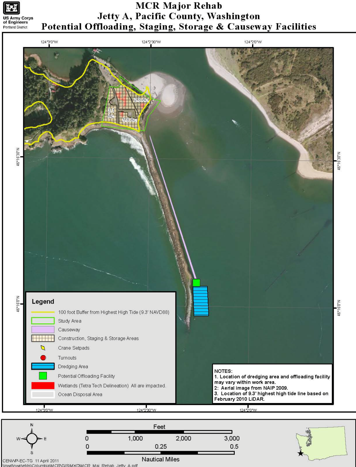
Figure 40. Jetty A Offloading, Staging, Storage and Causeway Facilities
