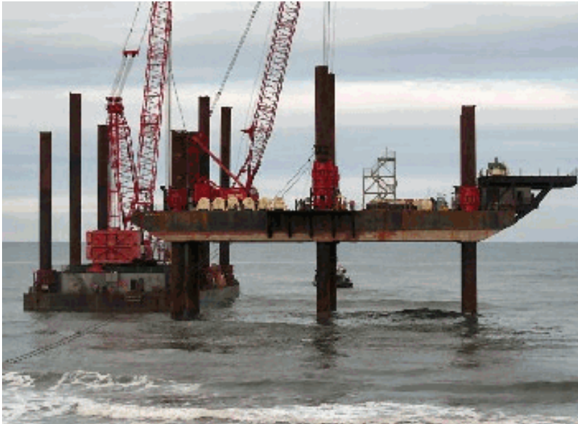
Figure 42. Illustration of a Jack-up Barge
