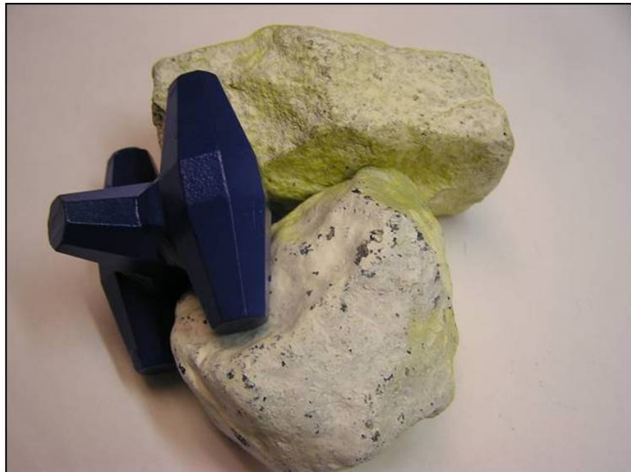
Figure A1- 175. Incompatibility Challenges between Concrete Armor Unit and Quarry Stone
