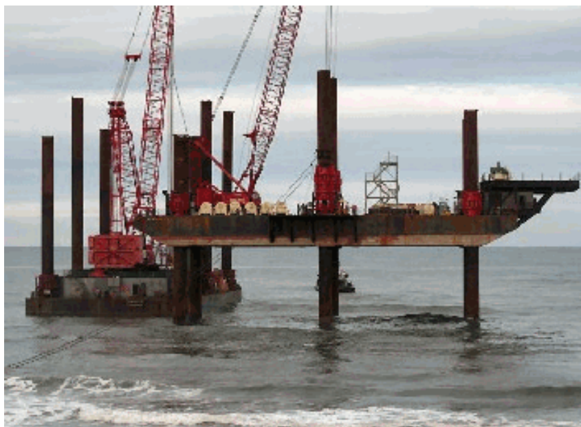
Figure 37. Illustration of a Jack-up Barge
