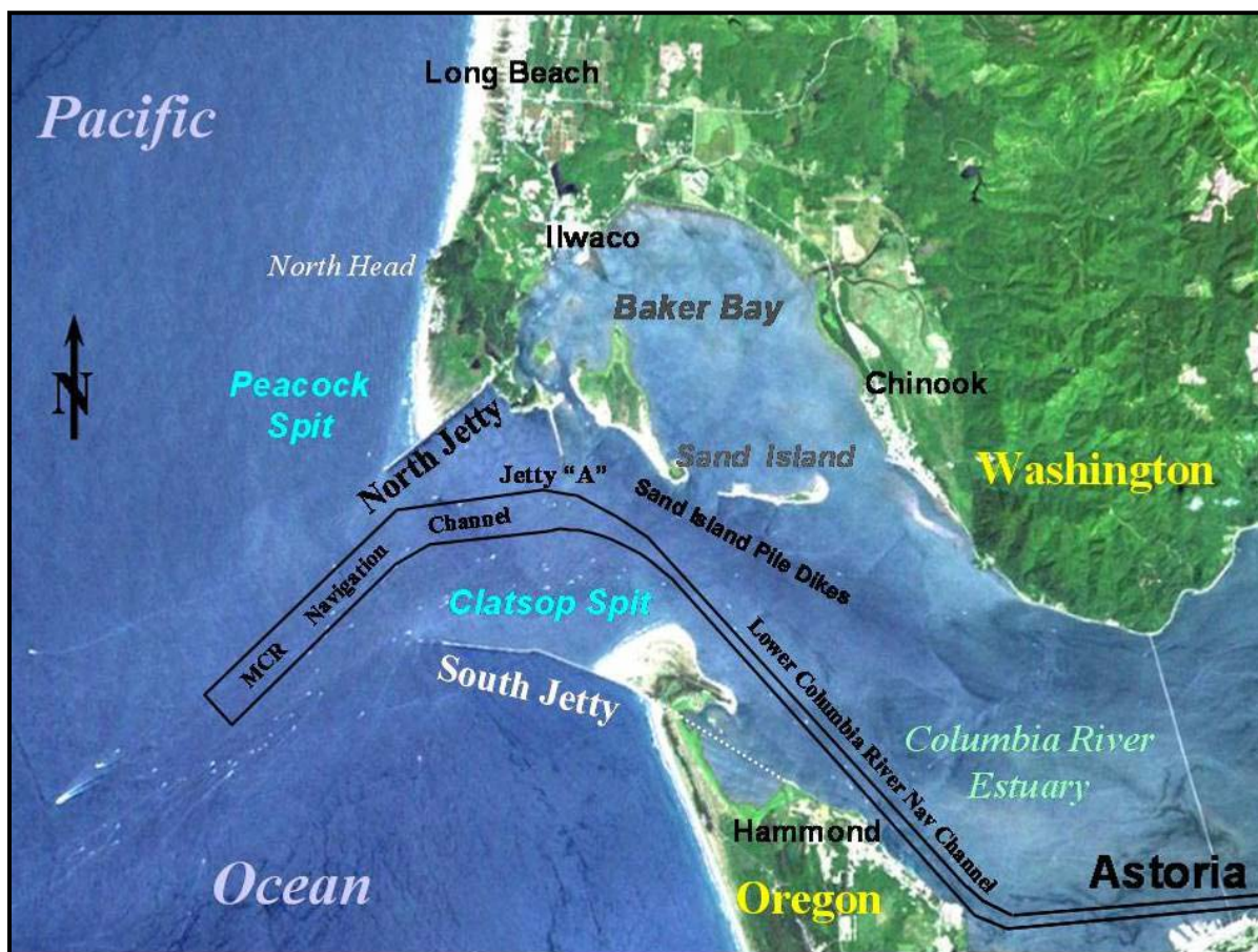
U.S. Army Corps of Engineers Jetty System at the Mouth of the Columbia River (MCR)
