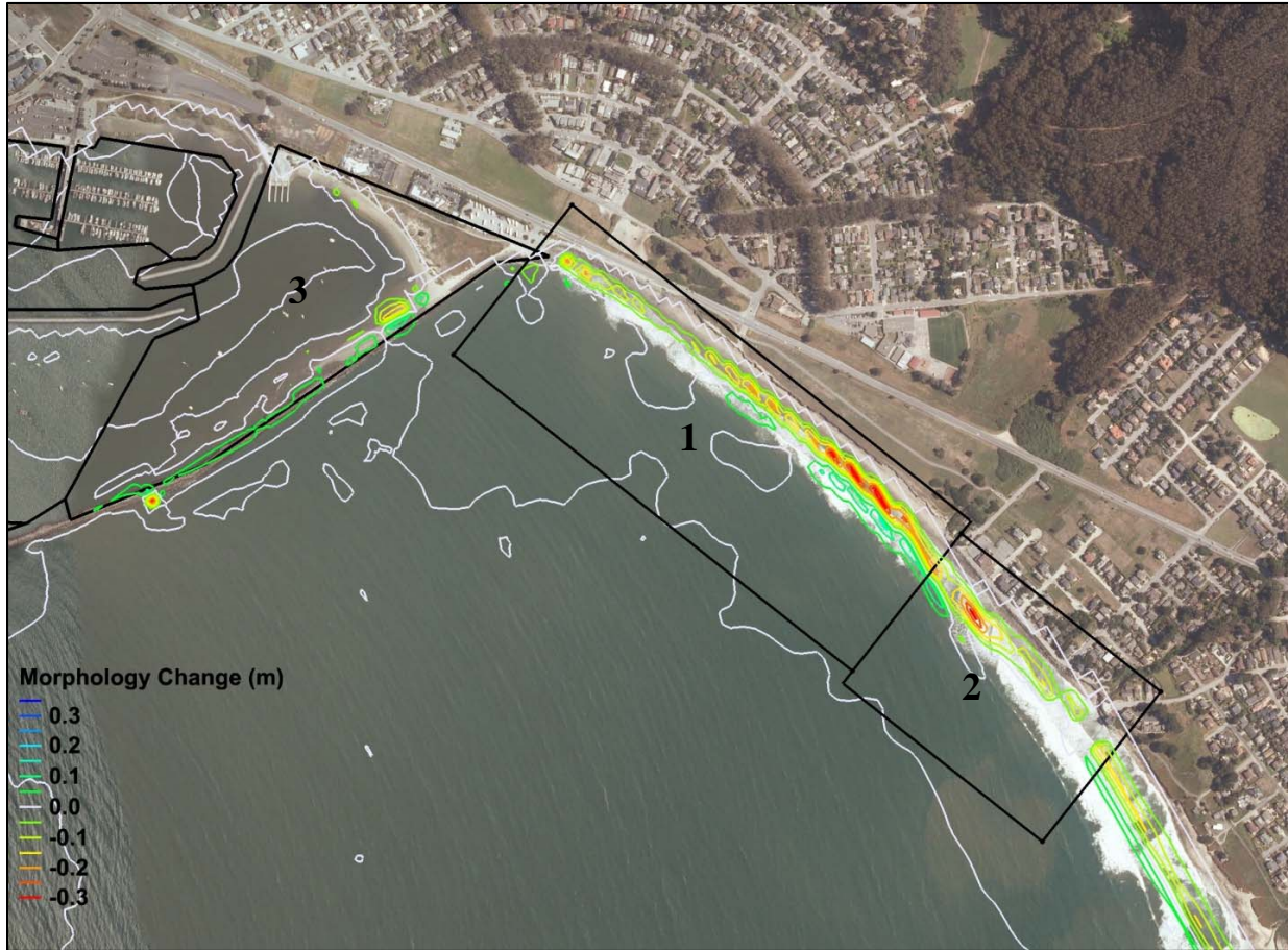
Figure 66. Morphology change associated with a breakwater notch from June to November 2009
