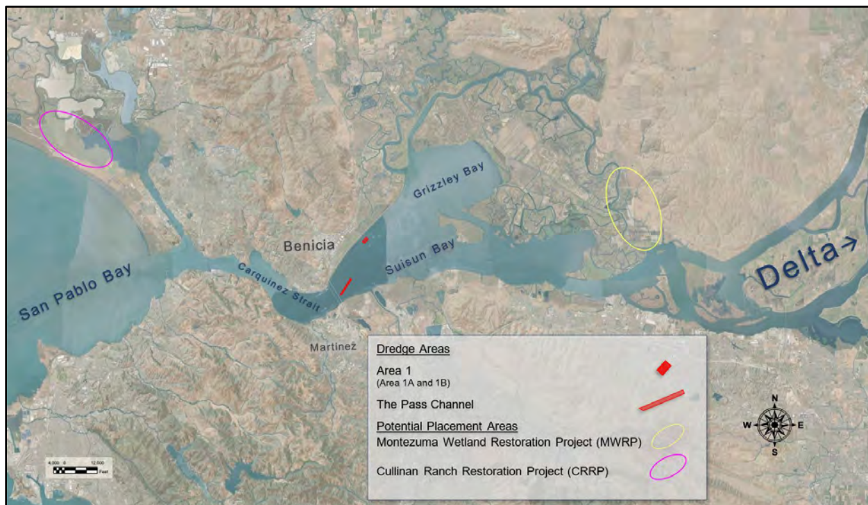
Figure 6: Suitable Beneficial Reuse Placement Sites.
