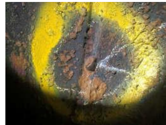
Typical Vertical Weld Pitting
