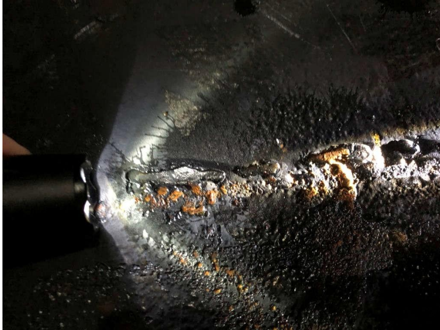
Photo A Typical Failed Coating on Bottom Welds
