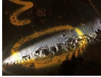
Bottom Butt-Weld Corrosion
