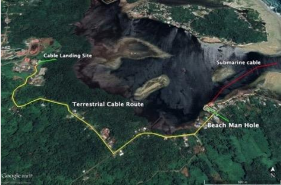
Figure 7: Proposed Terrestrial Cable Alignment
