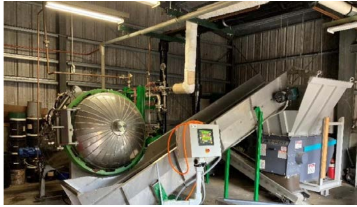
Newly installed and commissioned Rotoclave
