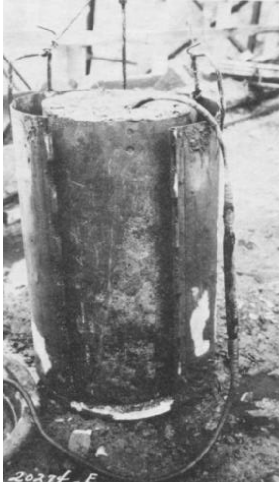
Figure C-8. No-Stress Meter Cylinder with Mold Partially Removed (courtesy of the Tennessee Valley Authority).
