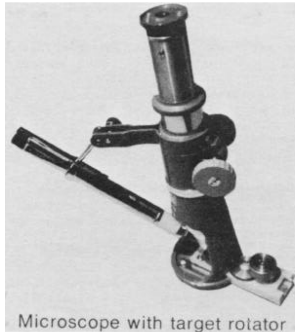
Figure 5-9. Scratch Strain Gage and Reading Microscope (Courtesy of Prewitt Associates).
