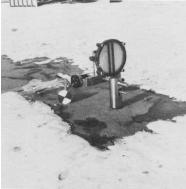
Figure 6-5. Inserted Micrometer Alignment Target. (Photo by WES)
