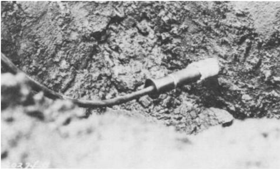
Figure C-14. Joint Meter Unit Screwed into Socket (Courtesy of the Tennessee Valley Authority).
