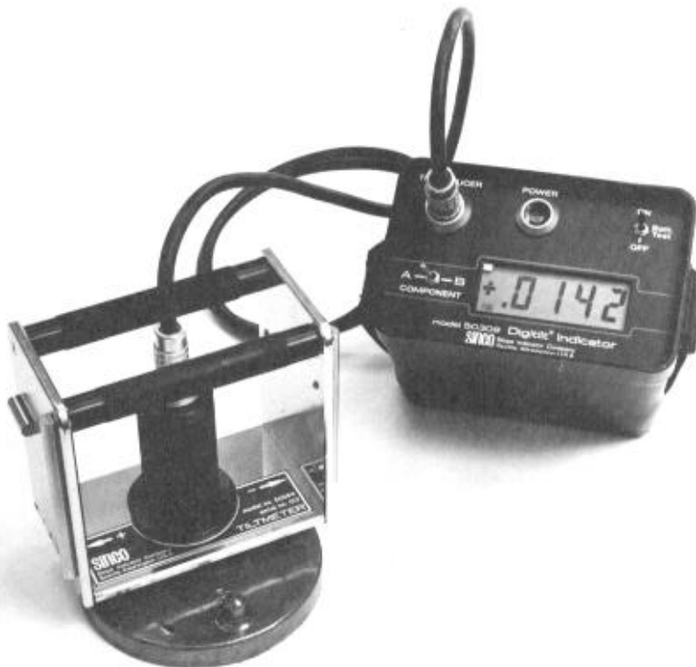
Figure 4-17. Portable Horizontal-Vertical Tiltmeter Sensor in Reading Position on Ceramic Tilt Plate
