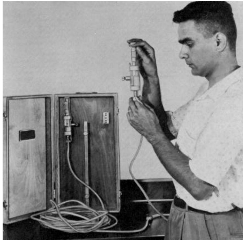
Figure 4-20. Autocollimating Tilt Measurement System
