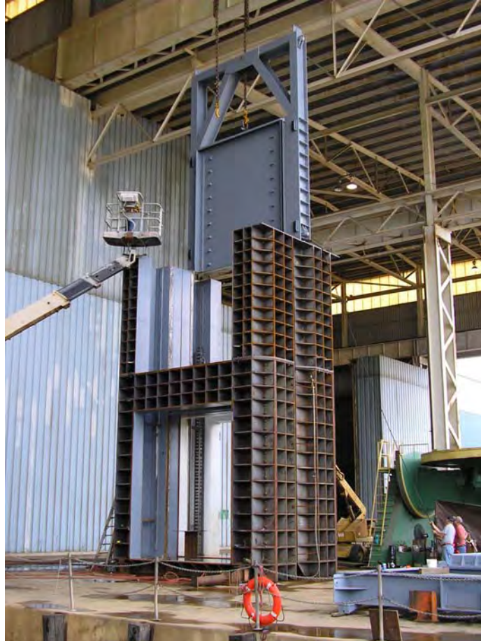
Figure 6-3. Stoney gate valve blade with liner
