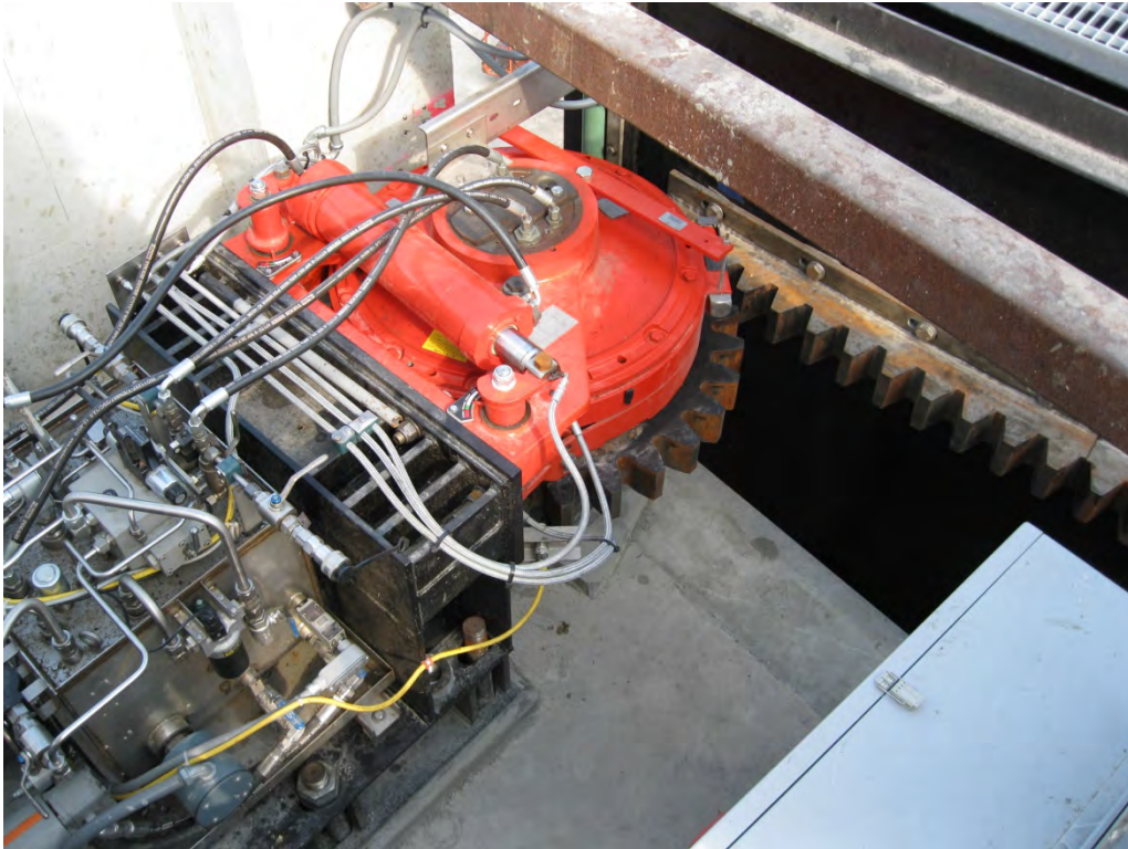
Figure 5-2. Hydraulically operated pinion gear and rack
