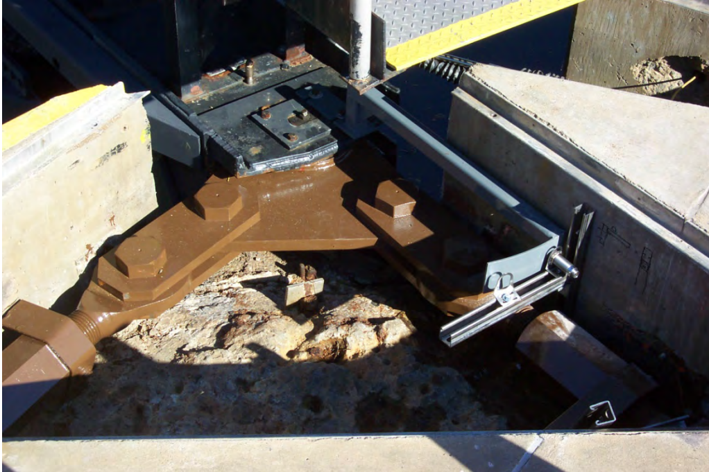
Figure 3-4. Moving target with multiple proximity sensors at gudgeon pin
