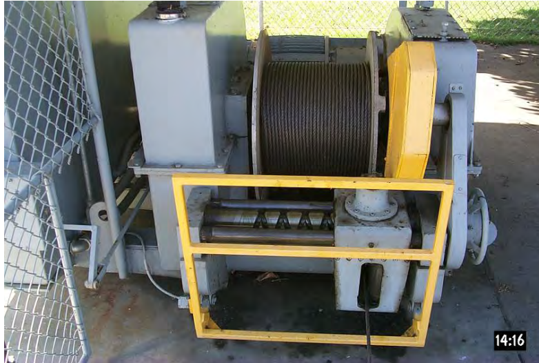
Figure 10-2. Mechanical winch unit with level wind system
