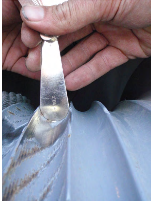
Figure 2-40. Checking wire rope drum groove profile
