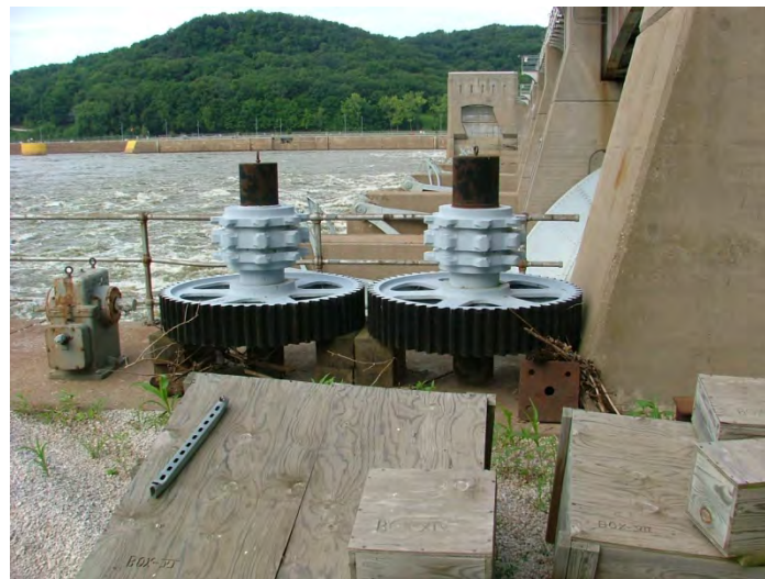
Figure 2-30. Dual chain pocket wheels with spur gear
