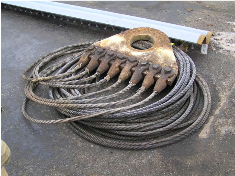
Figure 2-43. Multiple wire rope and vertical gate pin plate
