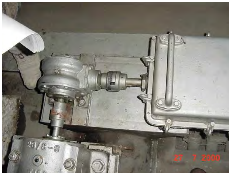
Figure 2-23. Jaw-type coupling detail
