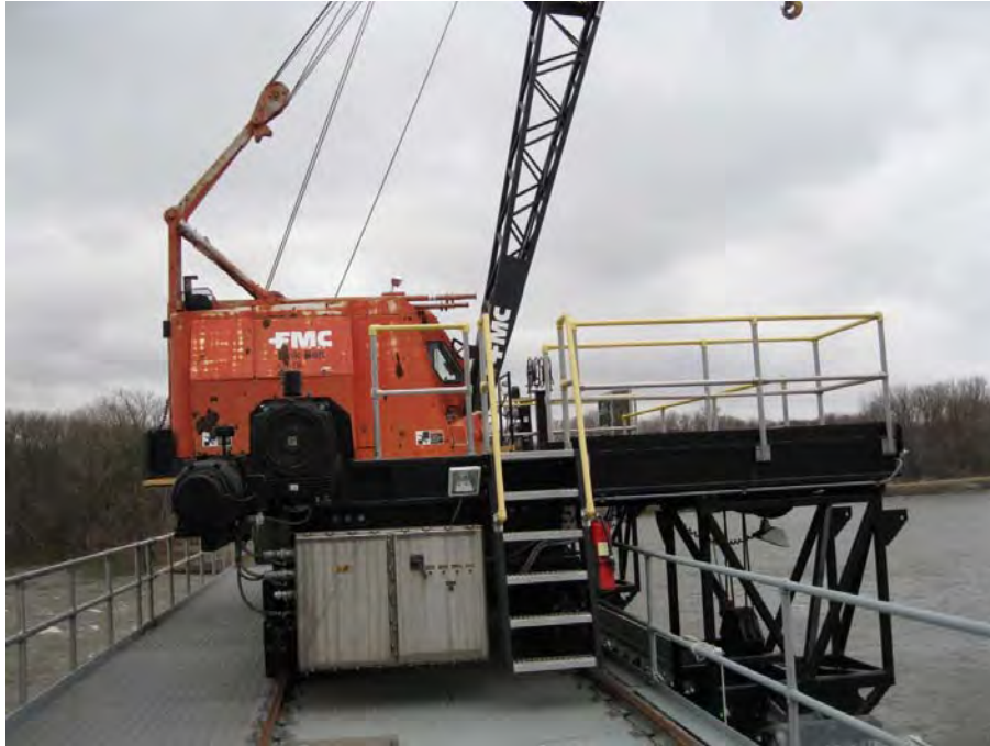
Figure 10-38. Bridge crane installed on an undercarriage
