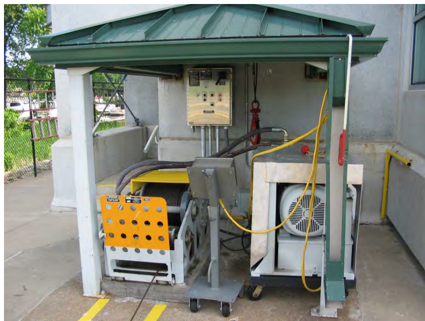
Figure 10-4. Hydraulic-operated tow haulage unit with level wind system
