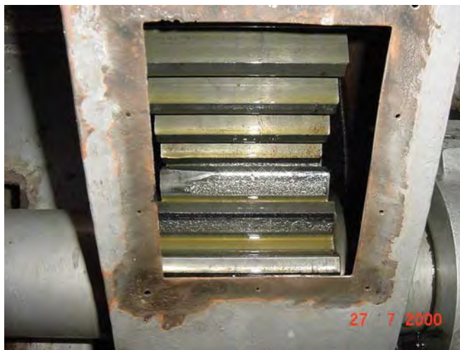
Figure 2-27. Oil bath spur gear with wear
