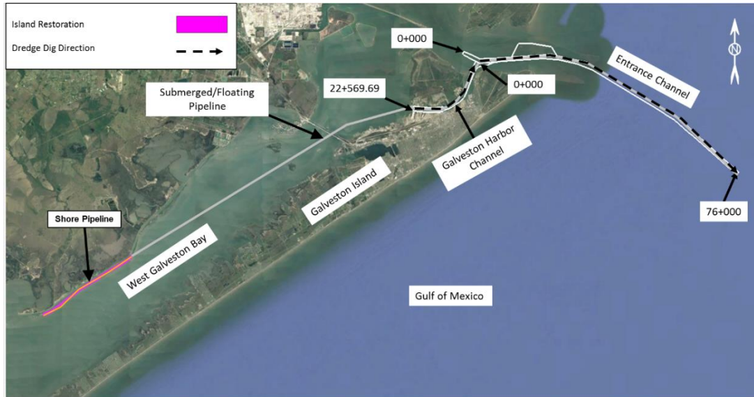
Figure 64. G -28 Island Creation and Restoration - 34” Hydraulic Direct Pump out
