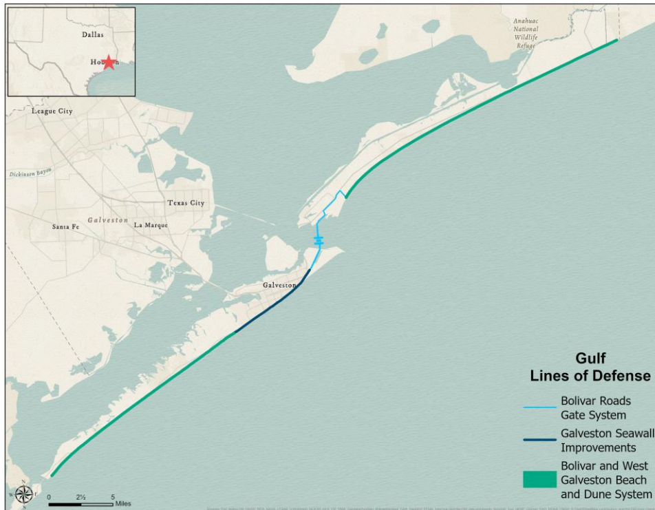
Figure 4. Galveston Bay Storm Surge Barrier System
