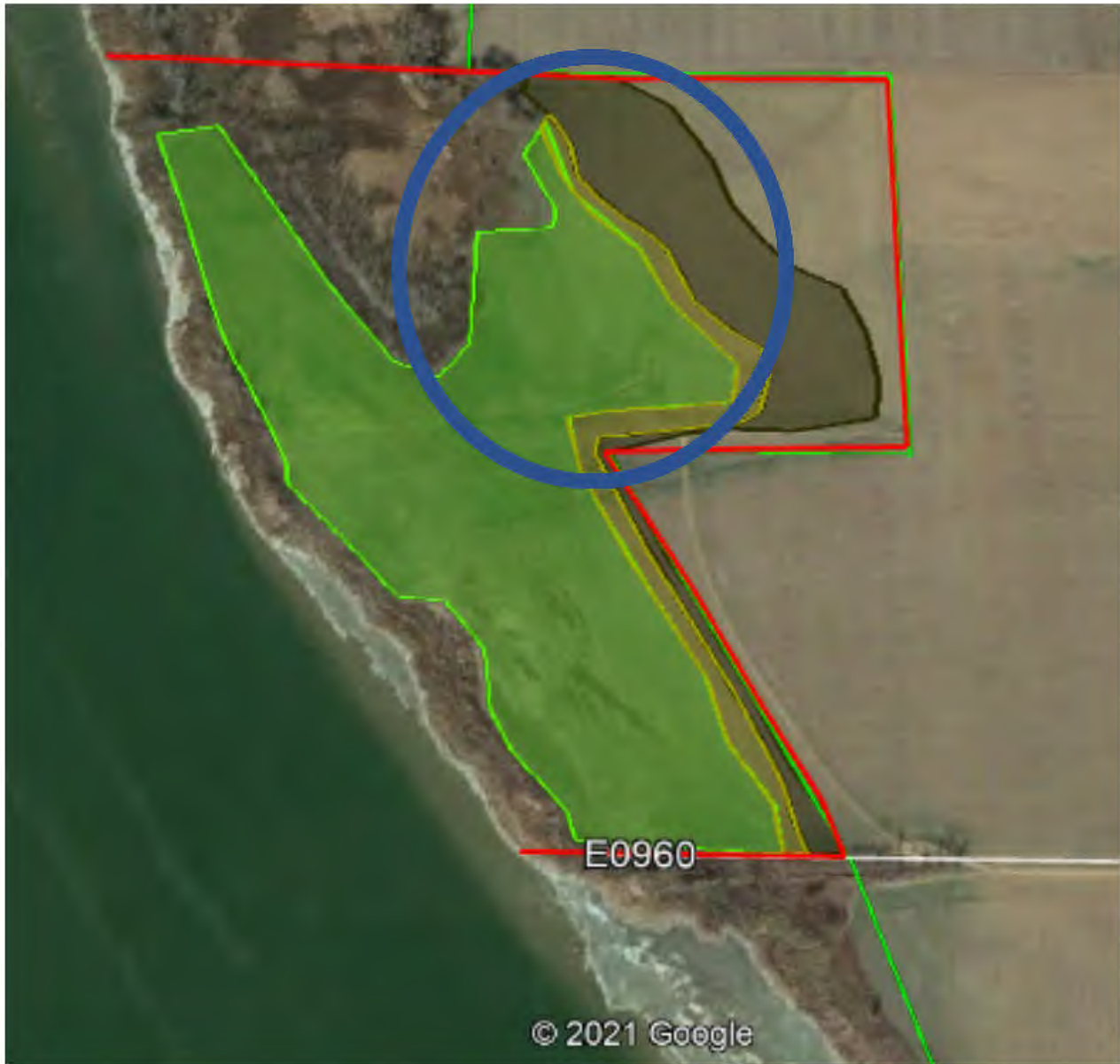
E0960: Grading in the area within the blue circle to match the rest of the green polygon. Approximate change in elevation between 4 to 9 feet. Approximately 1.0 miles of fencing.
