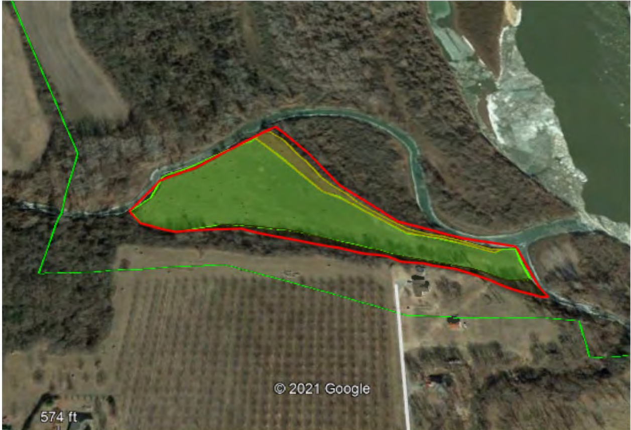
West Muskogee Turnpike: This site will need minor grading around the edges of the neon green polygon. There is a slight increase in elevation ~3 feet.
