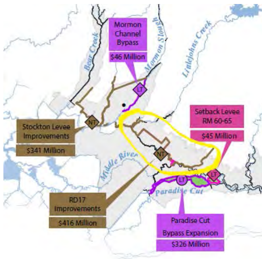
Figure 5. Elements of the State's Basin-Wide Feasibility Study tentative recommended plan in the vicinity of the proposed project include several regional options for habitat enhancement. Improvement to RD 17 with an additional setback area downstream of Middle River in lieu of fix-in-place improvement is highlighted (alignment offset within yellow circle).
