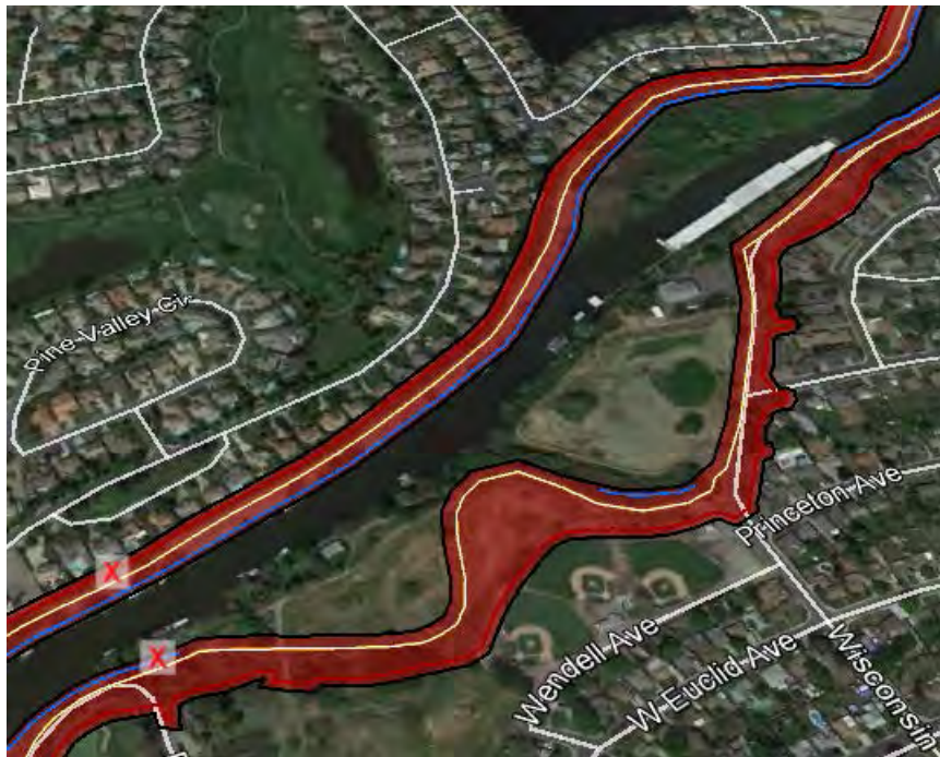
Figure 4. Location of existing set back area of levee on the right (south) bank of the Calaveras River recommended for consideration as SRA and riparian cover mitigation. Red shading is the extent of the existing levee profile plus maintenance easements.
