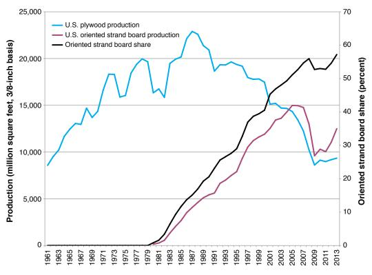
Figure 8—Production of plywood and oriented strand board in the United States, 1961-2013 (Sources: Adair 2010, APA 2014).
