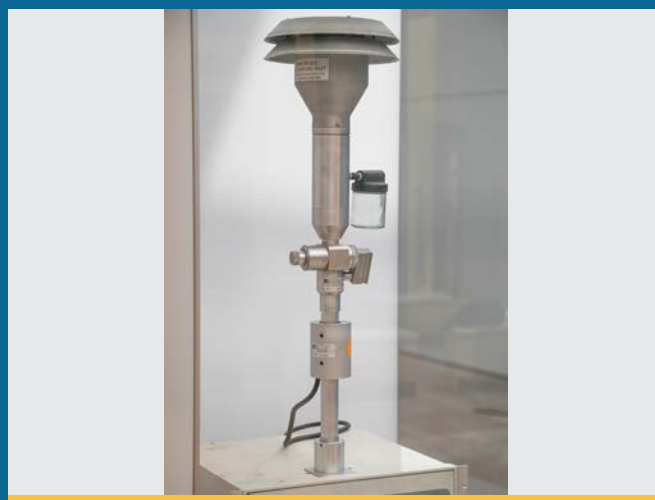
Original air quality monitoring device installed on the roof of the U.S. Embassy in Beijing in 2008. Instruments like this are now used at many U.S. embassies and consulates around the world to sample the air hourly and measure the level of particulate matter. Department of State
