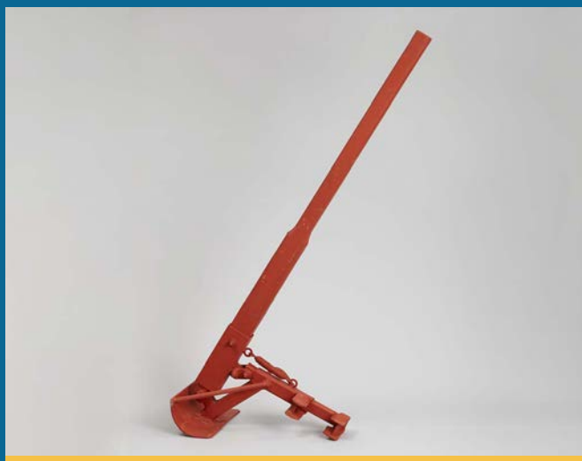
This unique object is a cococho: a tool used to uproot coca plants – the source of cocaine. State Department advisor Francisco “Paco” Alvarez developed the cococho in Peru in the late 1990s to eradicate coca plants in an environmentally friendly way. Its sharp teeth inspired its name cococho – the local word for crocodile. Department of State
