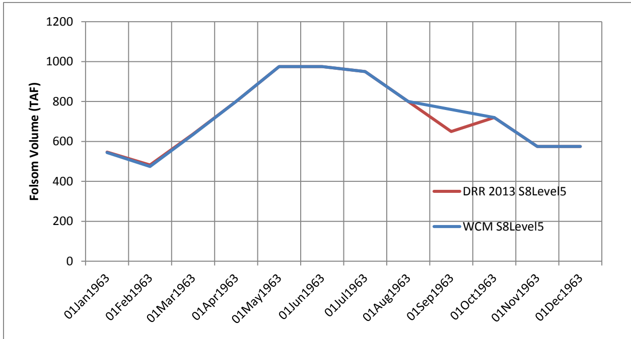
Figure 2-1. Comparison of Folsom Reservoir End-of-Month Flood Reservation Curve Volumes for the 2013 DRR and the Water Control Manual CalSim II Simulations.
