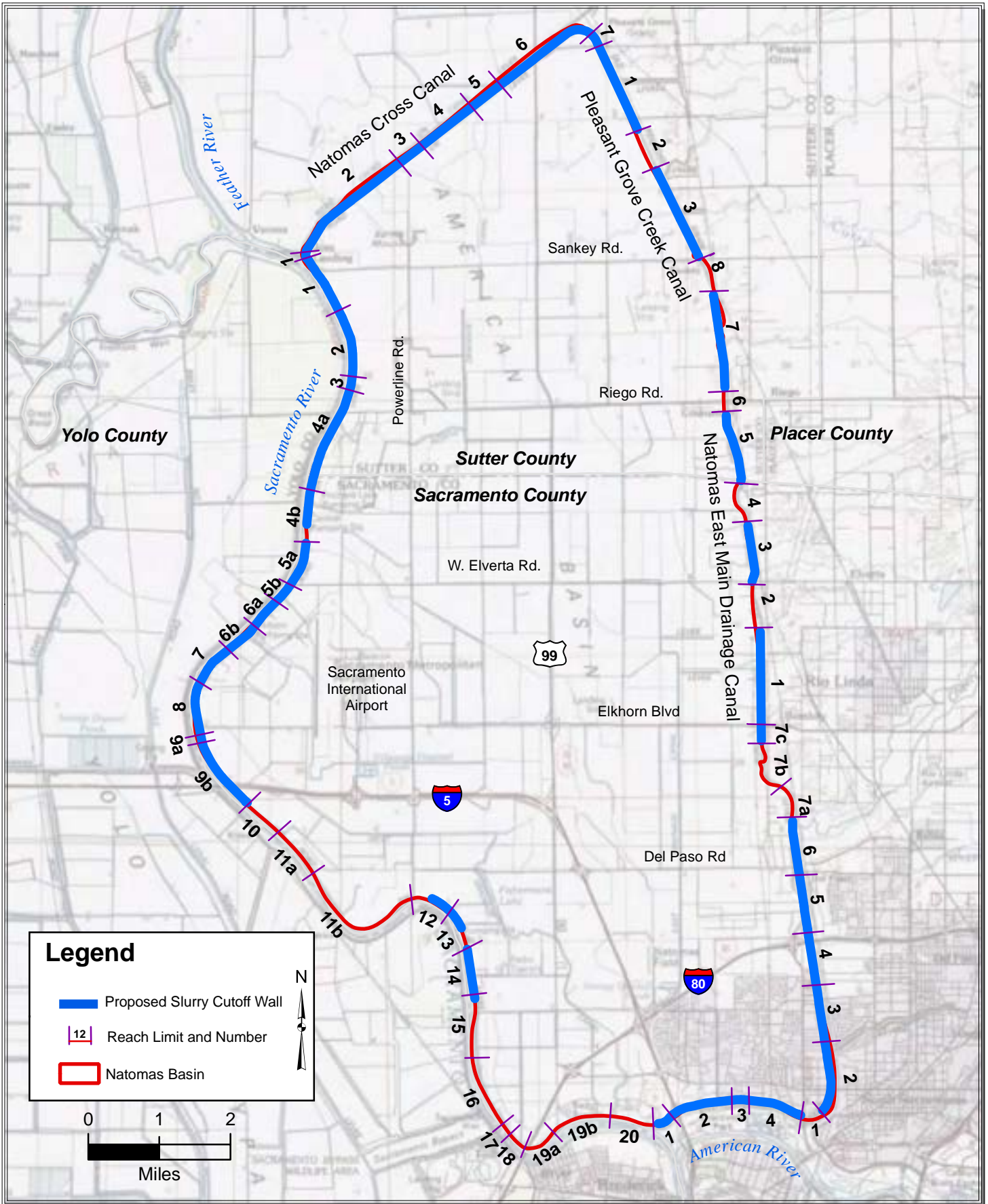
Figure 6-1 Proposed Slurry Cutoff Walls Surrounding Natomas Basin
