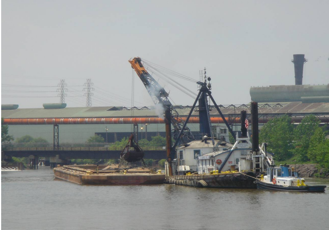
Figure 1.8 – Clamshell dredge loading a scow on the Upper Cuyahoga River
