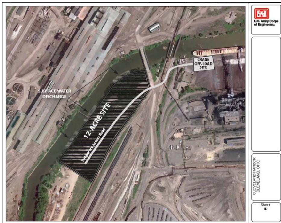
Figure 7-4. Conceptual design of offloading, dewatering, and re-handling facility for dredged material at the Upper River site.
