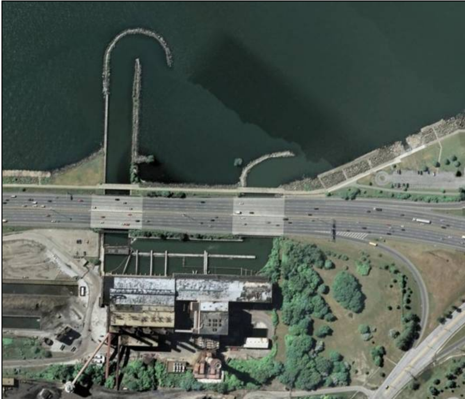
Figure 3-1. Google Earth snapshot of the First Energy Power Plant, thermal outfall (right) and cooling water intake (left) structures.
