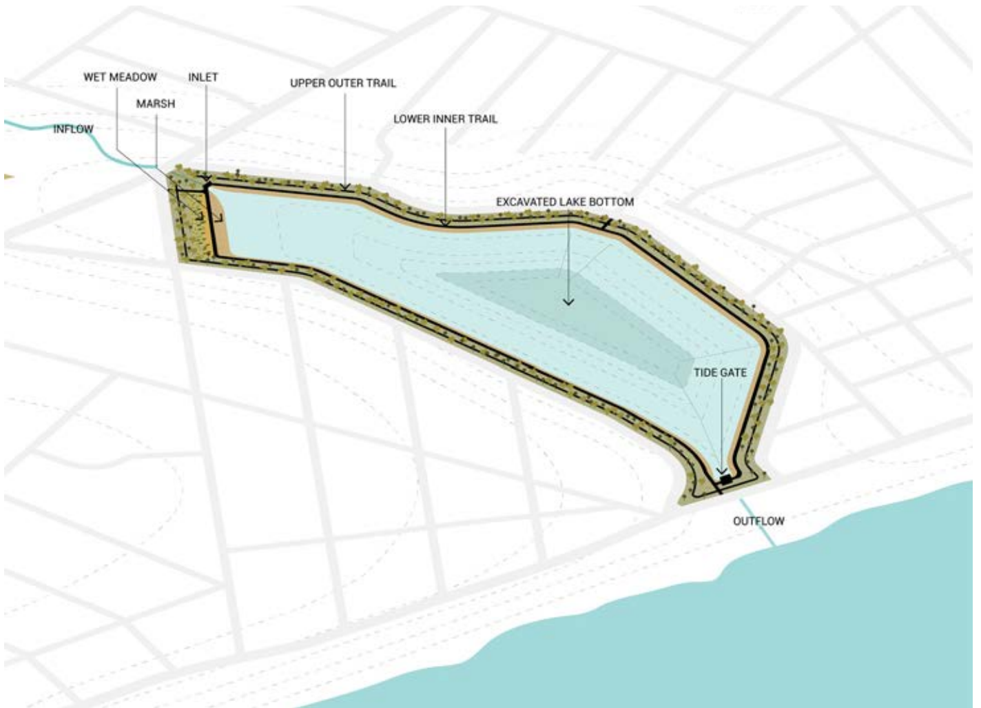
Diagrammatic vision for Lake Como with excavated lake bottom, terraced perimeter with planted ecological communities, and trails.
