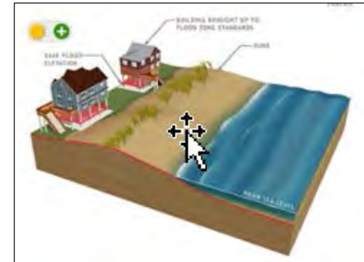
Building Retrofit including elevation
