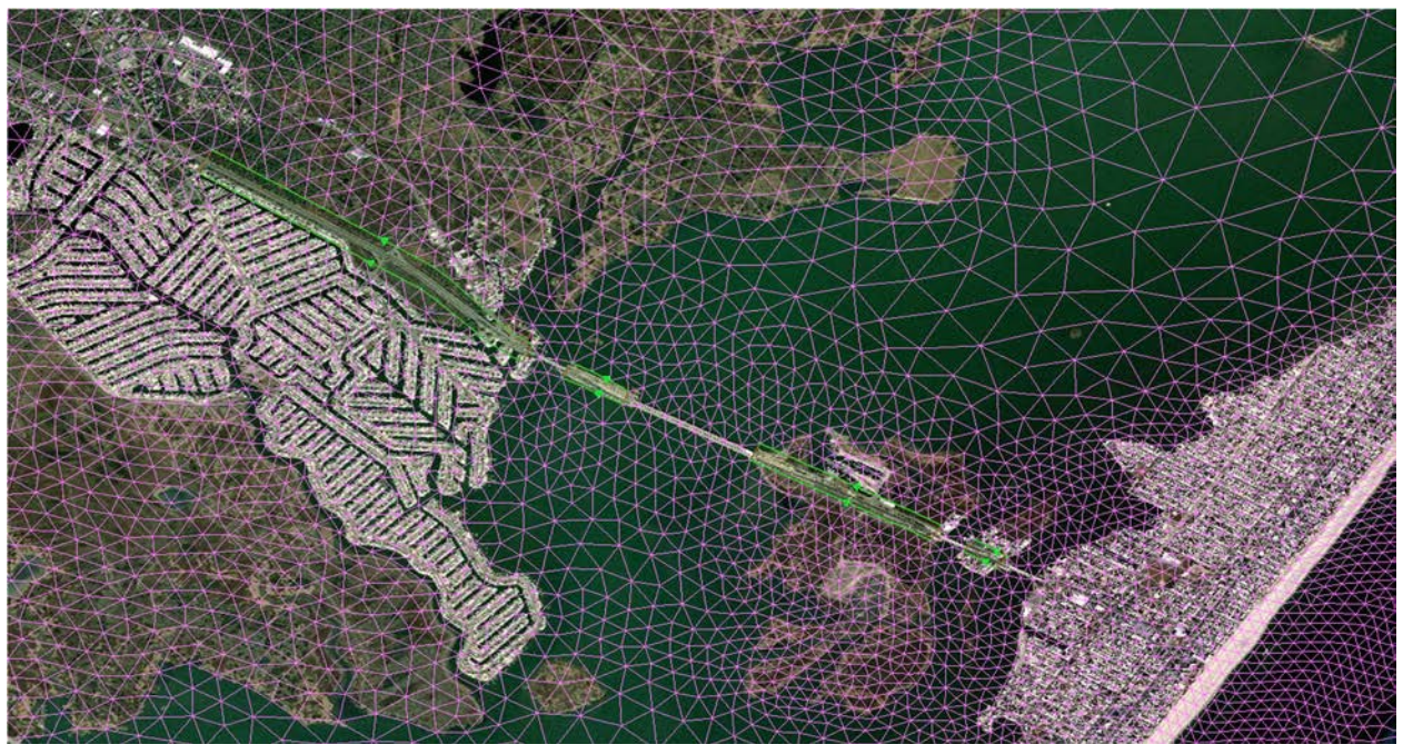
Figure 49: Rte. 72 Causeway - ADCIRC implementation
