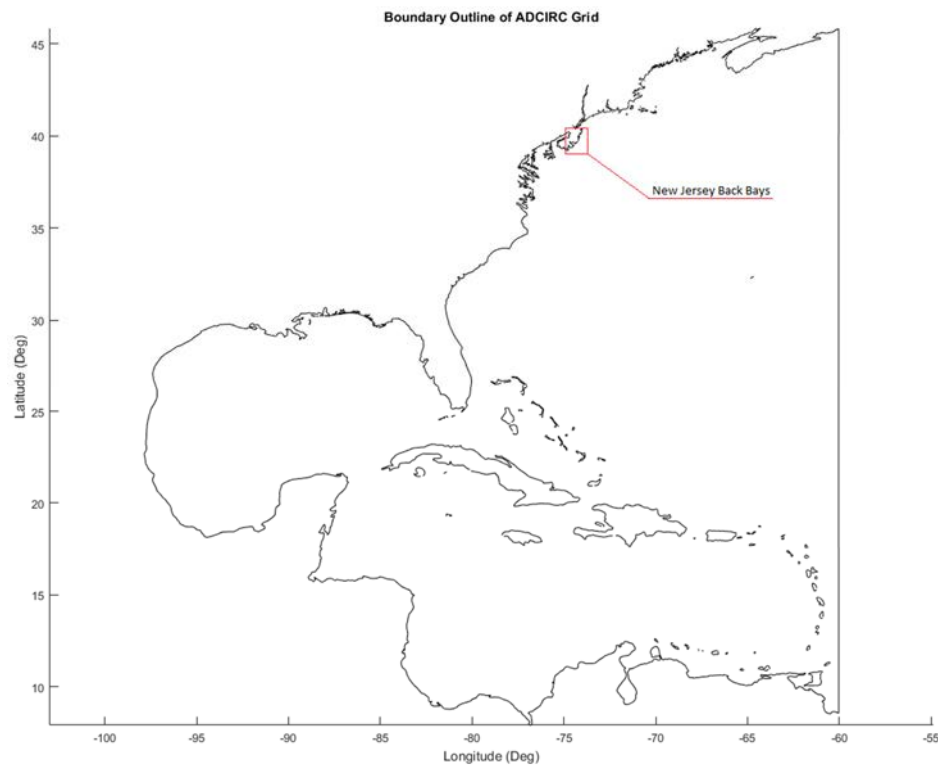
Figure 29: Outline plot showing the boundary of the ADCIRC grid.
