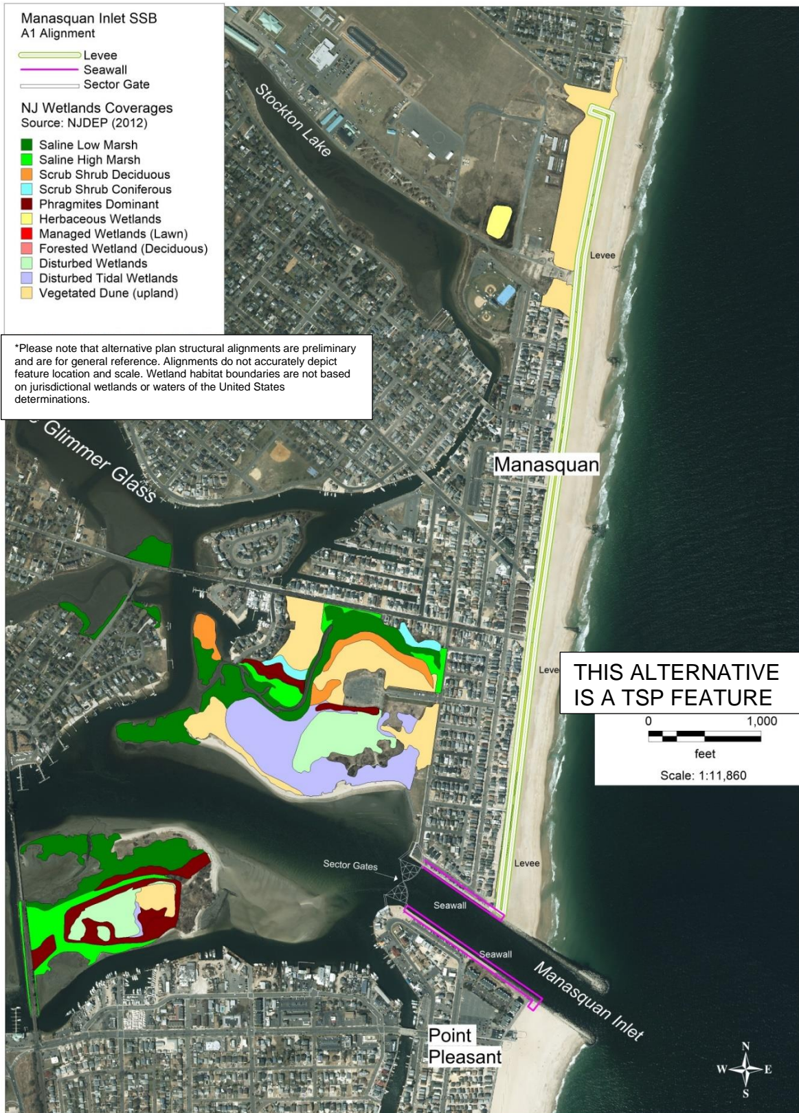
Figure 36. Storm Surge Barrier Overlay with Wetland Habitats at Manasquan Inlet in TSP Alternative 3E(2)
