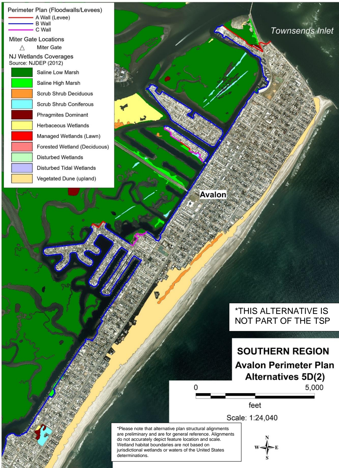
Figure 46. Perimeter Plan Overlay with Wetland Habitats along Avalon Alignment in Alternatives 5D(2).
