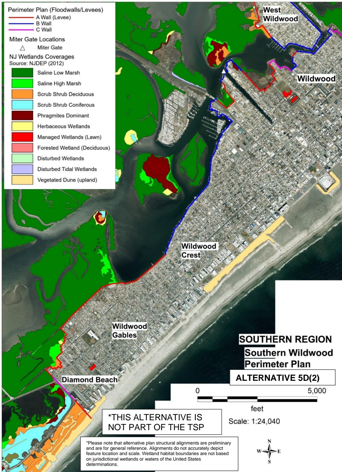
Figure 49. Perimeter Plan Overlay with Wetland Habitats along Wildwood (south) Alignment in Alternative 5D(2).
