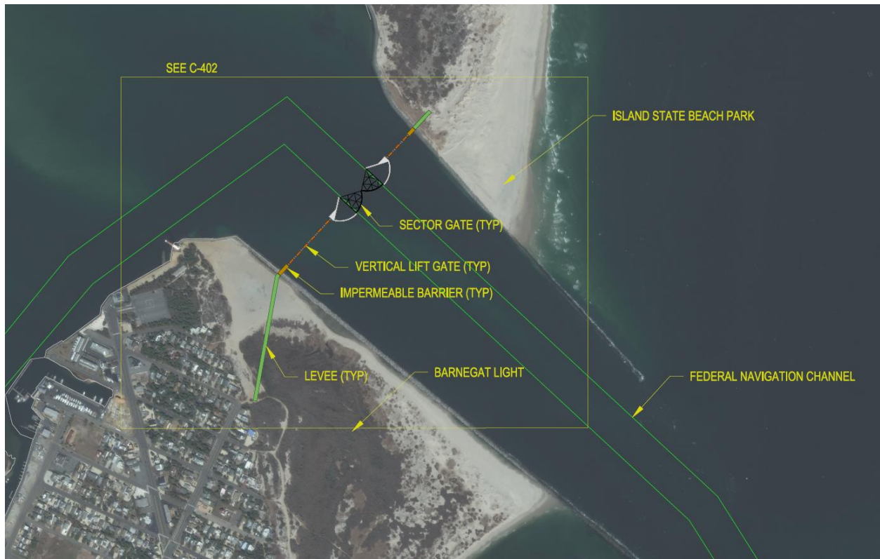
Figure 22: Storm Surge Barrier Example Design – Barnegat Inlet
