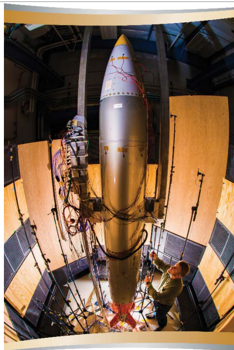
Sandia National Laboratory mechanical engineer adjusts a microphone for an acoustic test on a B-61-12 system.
