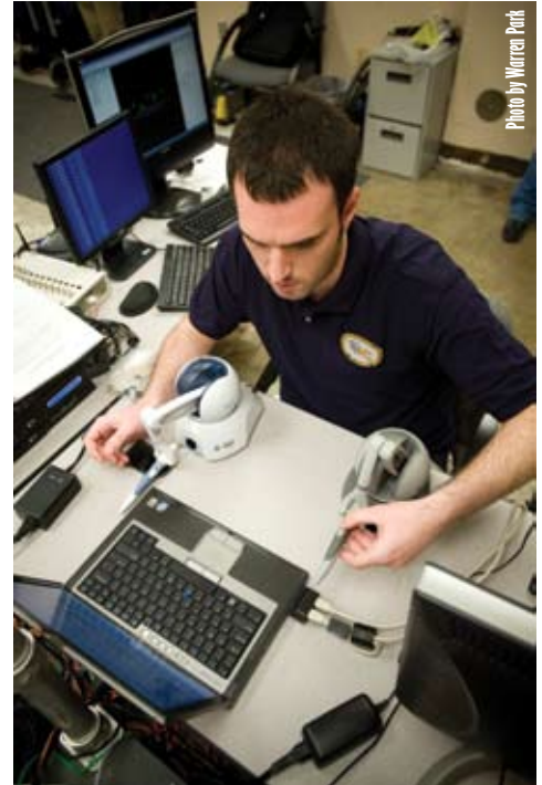
Engineer Juan Vazquez remotely operates the robotic arms on the perMMA as he views the user's surroundings, via wheelchair-mounted webcams, on a computer screen.
