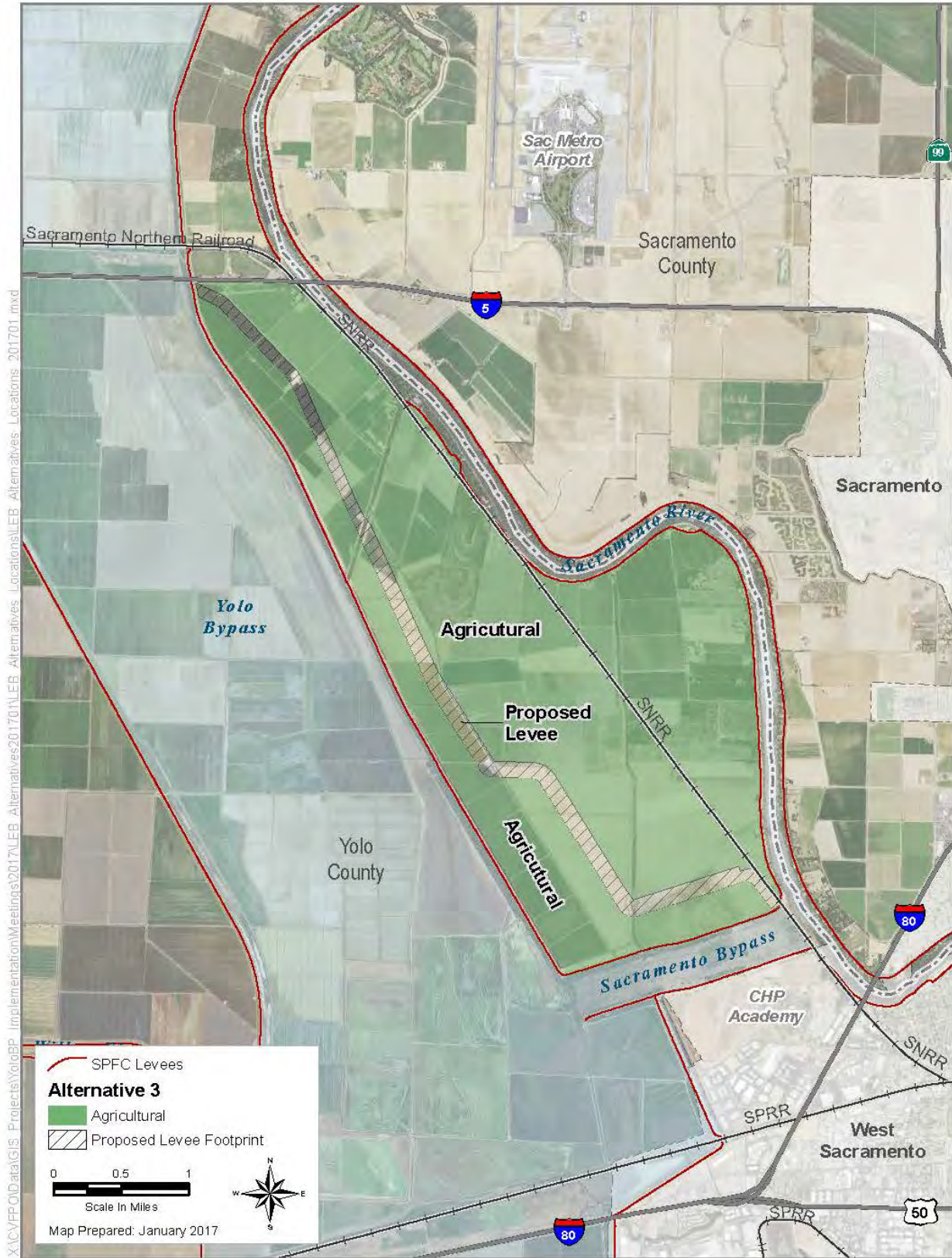
Figure 5. Alternative 3 Levee Setback Alignment
