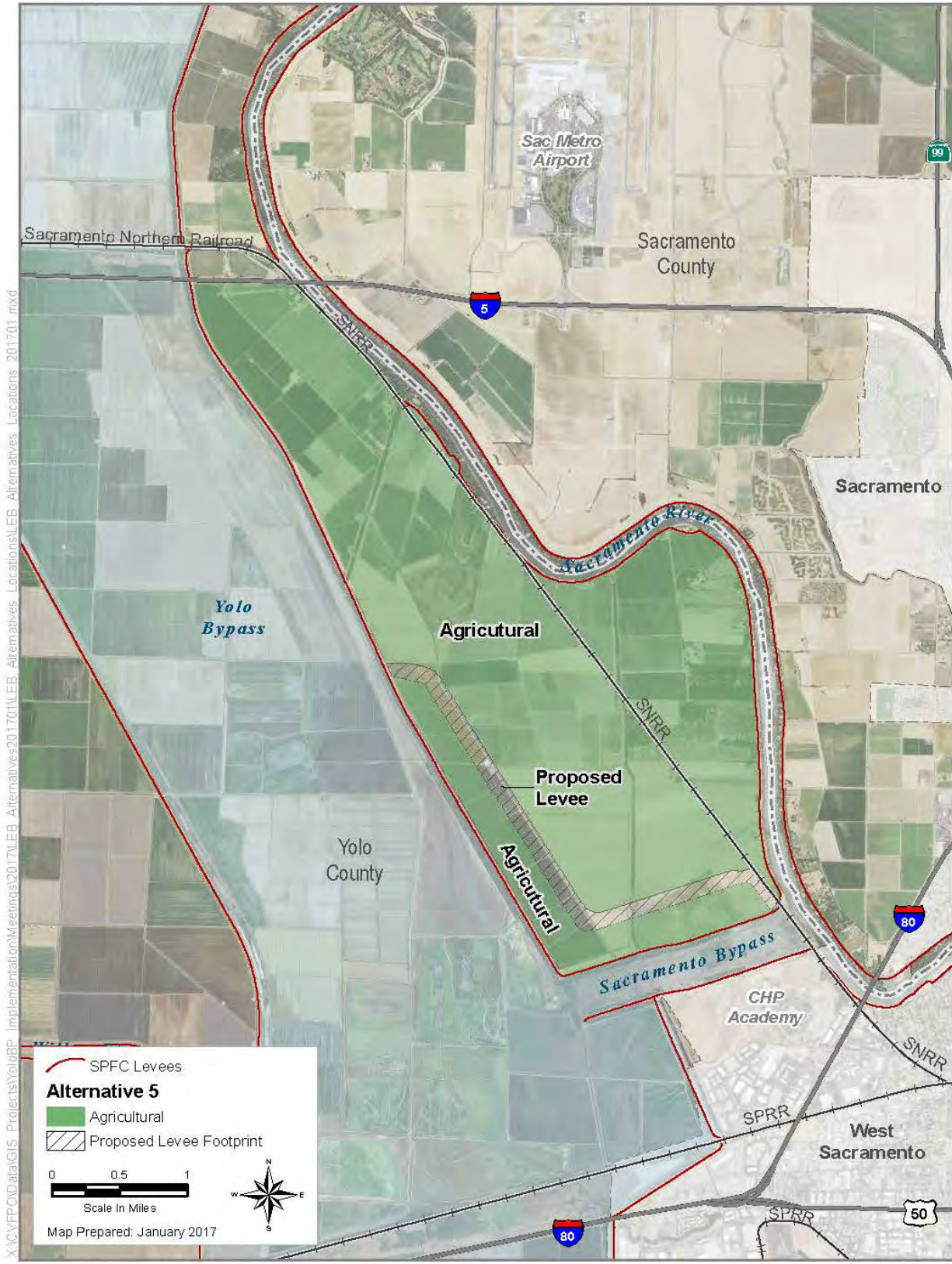
Figure 7. Alternative 5 Levee Setback Alignment
