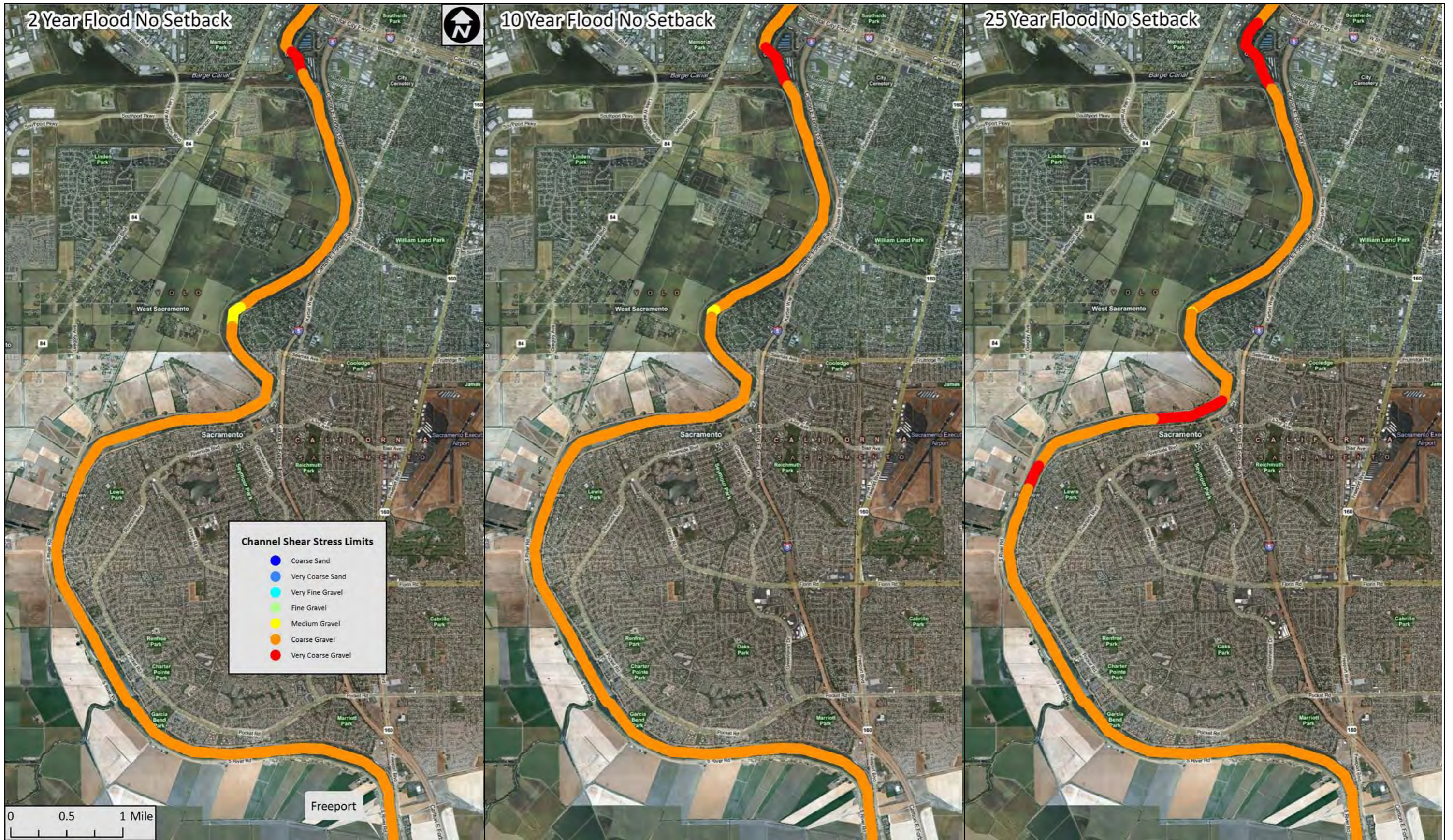
Shear stress limits based on Fischenich, 2001. Colors represent upper limit of shear stress power. Orthoimagery courtesy of Bing Maps.
