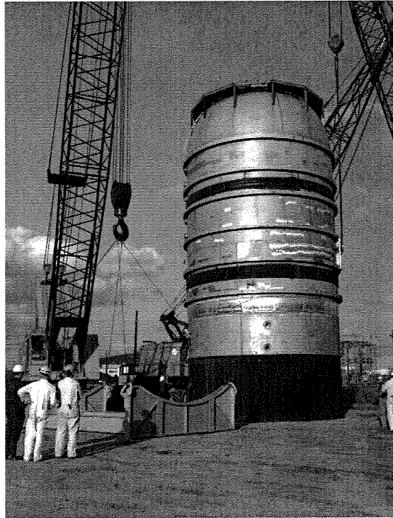
Plate 11: Battleship S-IVB at the S-IVB Stage Test Facility (Douglas Missile Test Facility), 1 February 1965. Marshall Space Flight Center MIX Archives.
